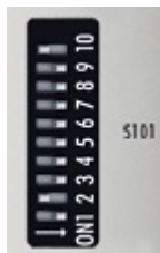
Abb. 14: DIP-Schalter S001: Links off "0", rechts on "1"
