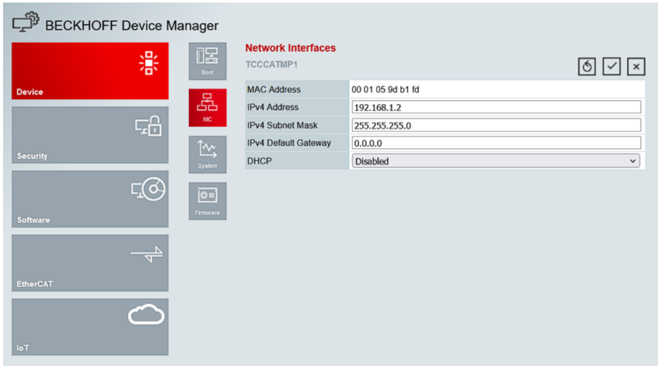
Fig. 34: Beckhoff Device Manager Device - NIC
