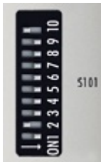
Abb. 13: DIP-Schalter S001, Links off "0", rechts on "1"
