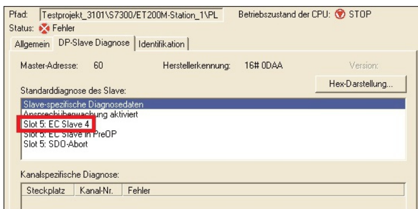
Fig. 23: Diagnostic example via PROFIBUS with a Siemens project configuration.
