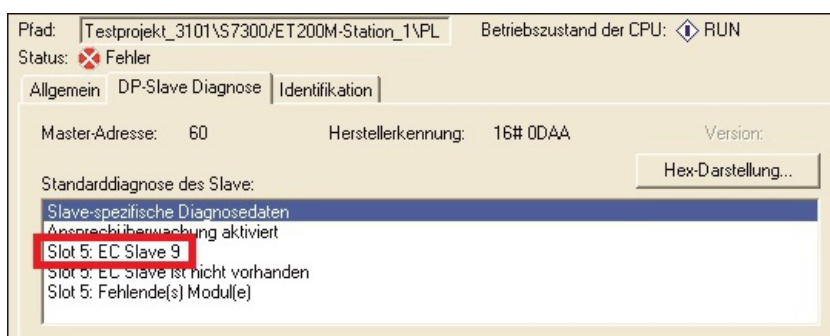
Fig. 24: Diagnostic example via PROFIBUS for virtual slaves with a Siemens project configuration.
