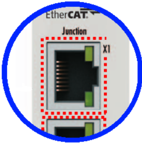
Fig. 5: Fast-Hot-Connect ports at the EK1122-0080
