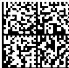
Fig. 3: Example DMC 1P072222SBTNk4p562d71**KEL**1809 Q1 **51S**678294
