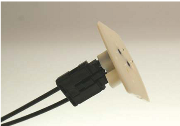
Fig. 58: Sanding gauge with protruding fiber ends
