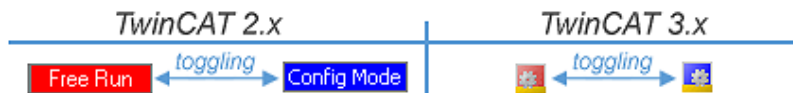
Fig. 111: Displaying of “Free Run” and “Config Mode” toggling right below in the status bar
