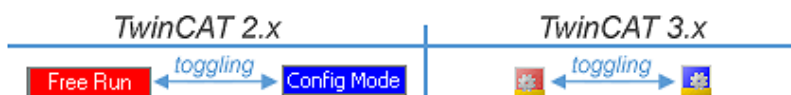
Fig. 97: Displaying of “Free Run” and “Config Mode” toggling right below in the status bar
