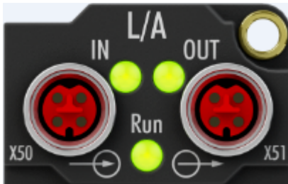
Fig. 22: EtherCAT P-Box, Connectors for EtherCAT P
