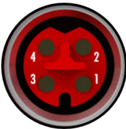
Fig. 23: Pin assignment M8, EtherCAT P In and EtherCAT P Out
