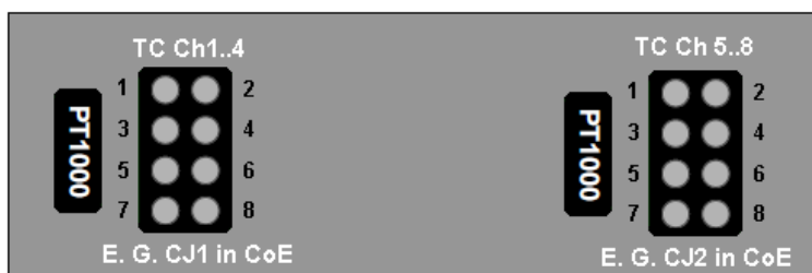
Fig. 23: Routing of the TCs to two different TC connectors using the example of EJ3318
