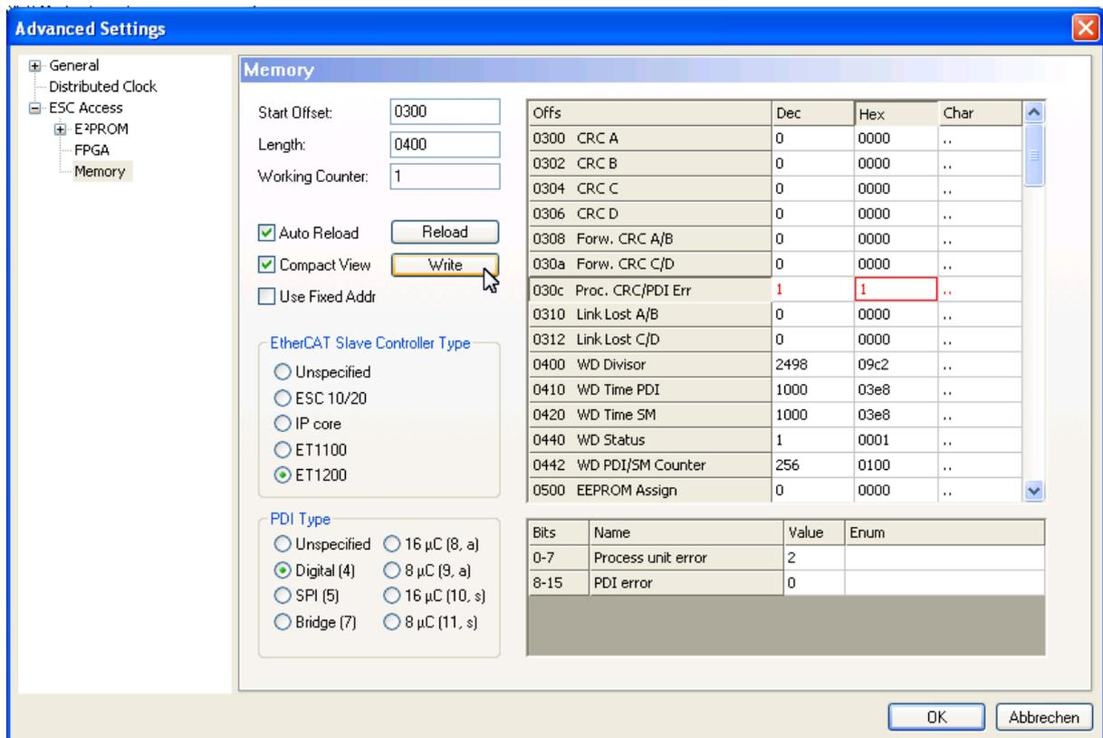
Figure 27: Write to the error counter to clear it
