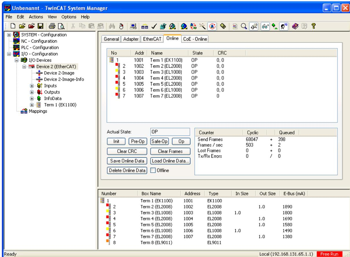
Figure 17: TwinCAT logging CRC error counters
