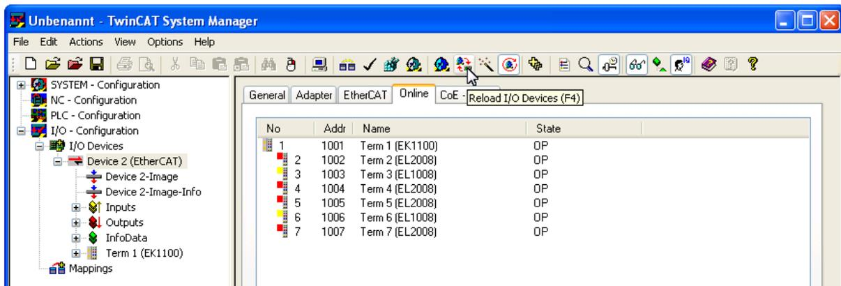
Figure 20: Reload I/O Devices (F4) after disabling CRC logging
