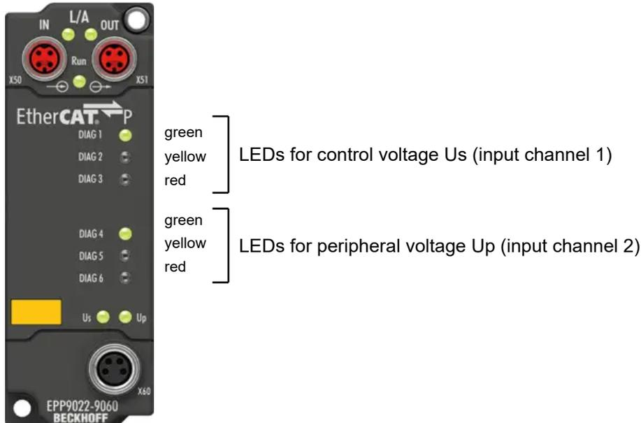
Fig. 7: Assignment of the LEDs
