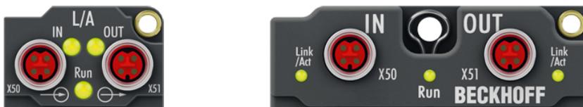
Fig. 5: Connectors for EtherCAT P
