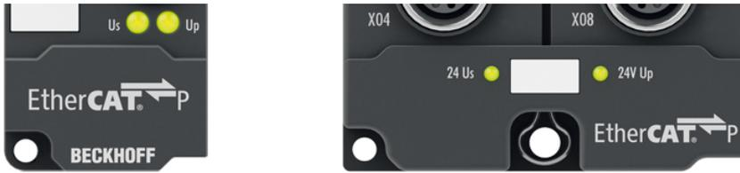
EtherCAT P Box modules indicate the status of the supply voltages via two status LEDs. The status LEDs are labeled with the designations of the supply voltages:  $U_s$  and  $U_p$ .
