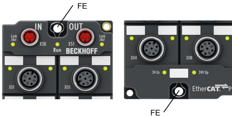
Fig. 2: Connection for functional earth (FE)
