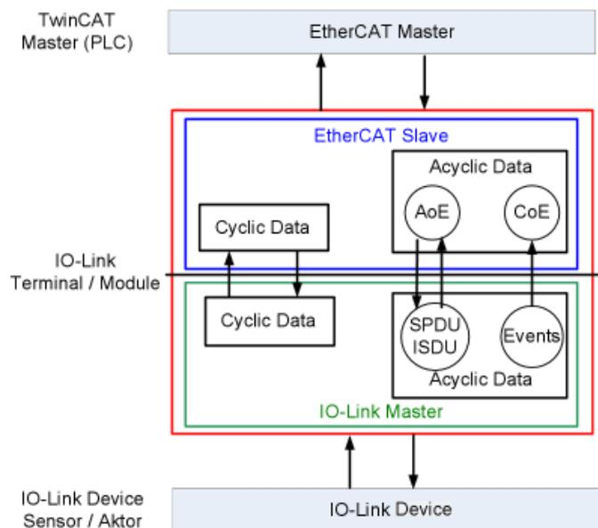
Fig. 36: Illustration of the system communication of an EtherCAT master
