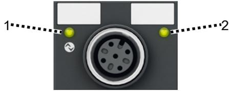
Fig. 6: Status LEDs of an IO-Link port
