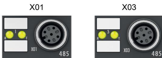
Abb. 9: RS422 / RS485 Status-LEDs
