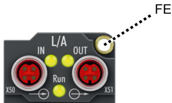
Fig. 8: Connection for functional earth (FE)
