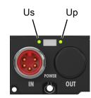
A status LED lights up if the corresponding voltage is present and correctly connected.
