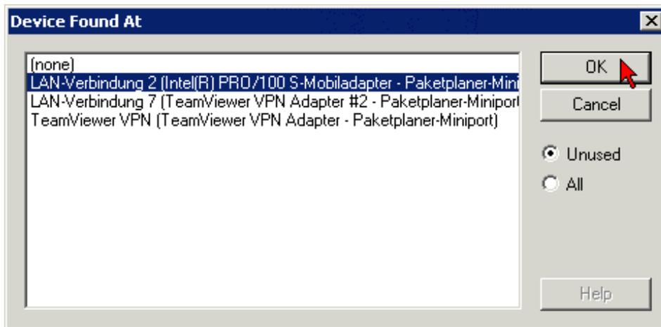
Fig. 24: Selection and confirmation of the Ethernet adapter
