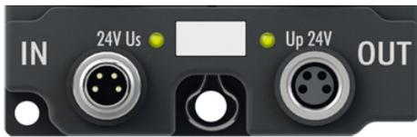
Fig. 13: Connectors for supply voltages
