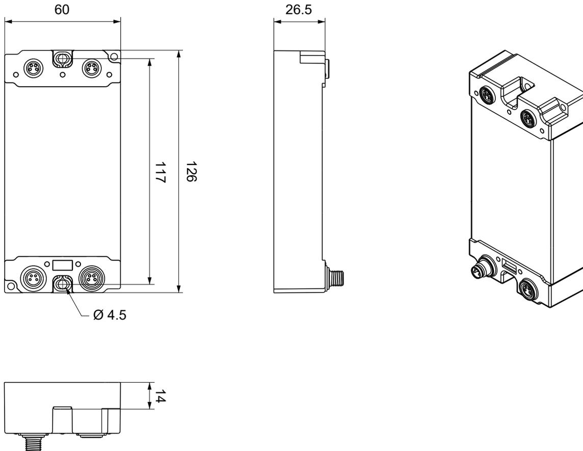
All dimensions are given in millimeters.
