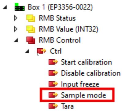
Fig. 9: Sample mode switching
