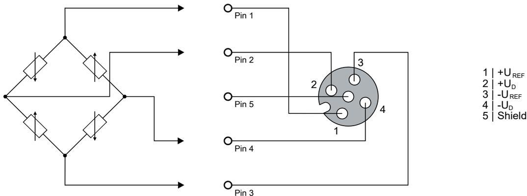
Connect the cable shield to pin 5 of the M12 connector.
