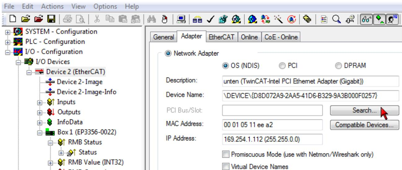
Fig. 23: Searching the Ethernet adapter
