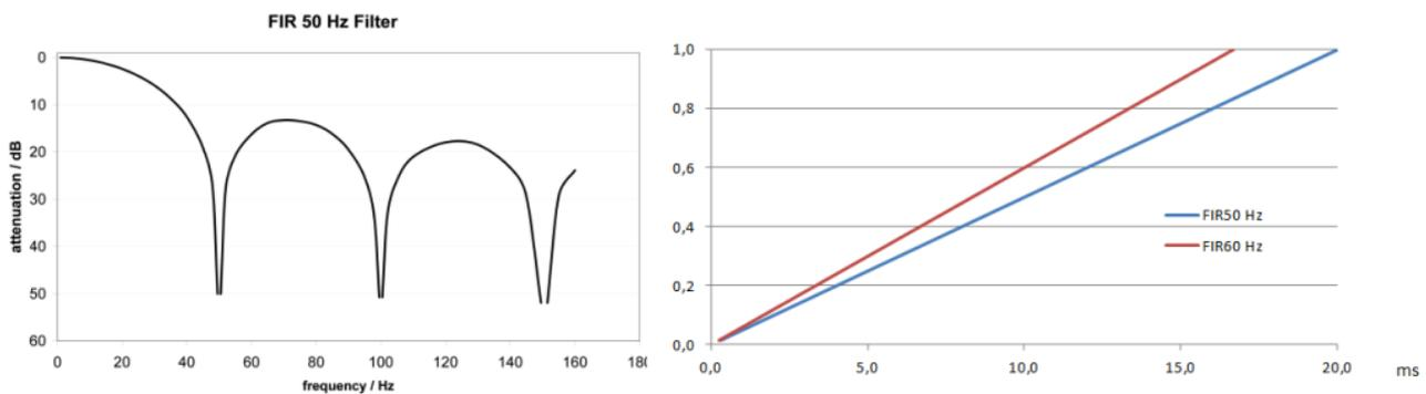
Fig. 4: Notch characteristic/amplitude curve and step response of the FIR filter
