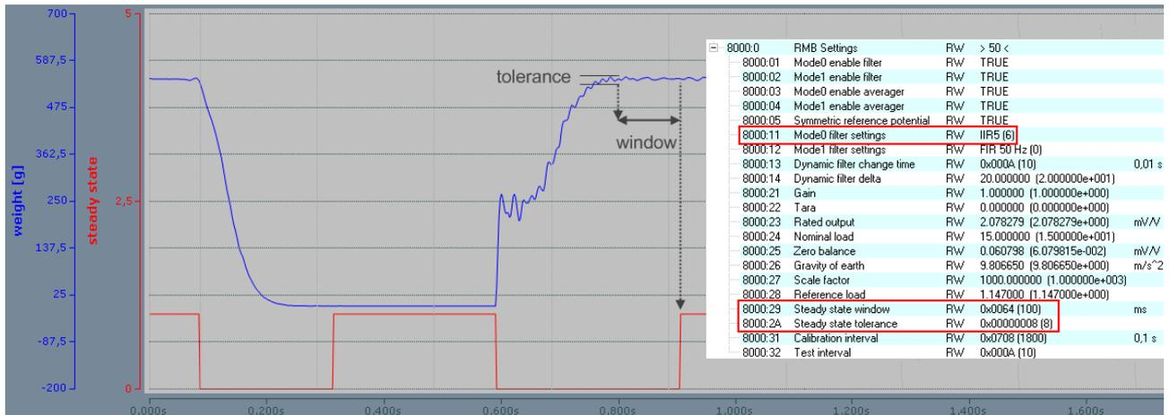
Fig. 19: Abrupt unloading and subsequent reloading of a load cell
