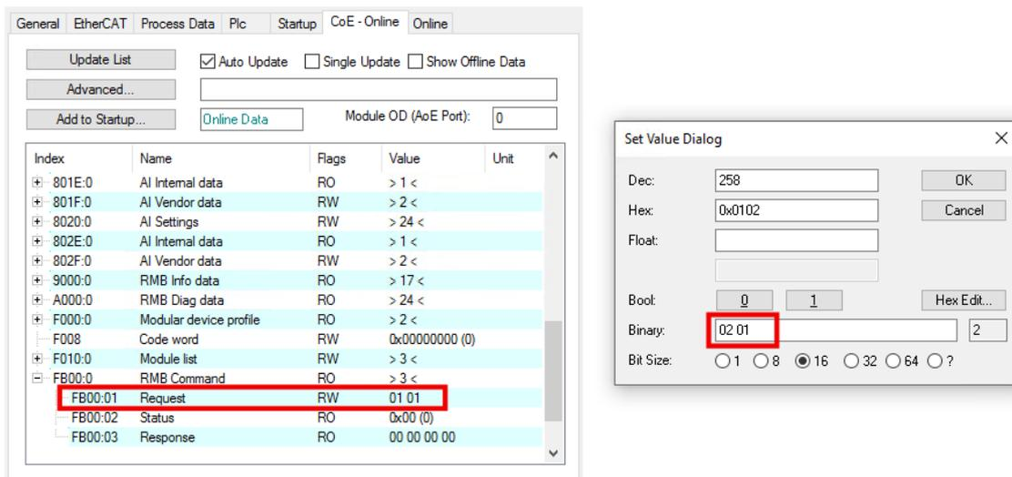
10. Reset: execute the command "0x0000" (0<sub>dec</sub>) on CoE object 0xFB00:01 [▶ 63].
