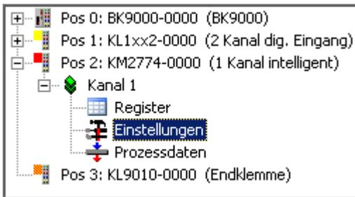
Fig. 7: KS2000 branch for channel 1 of the KM2774
