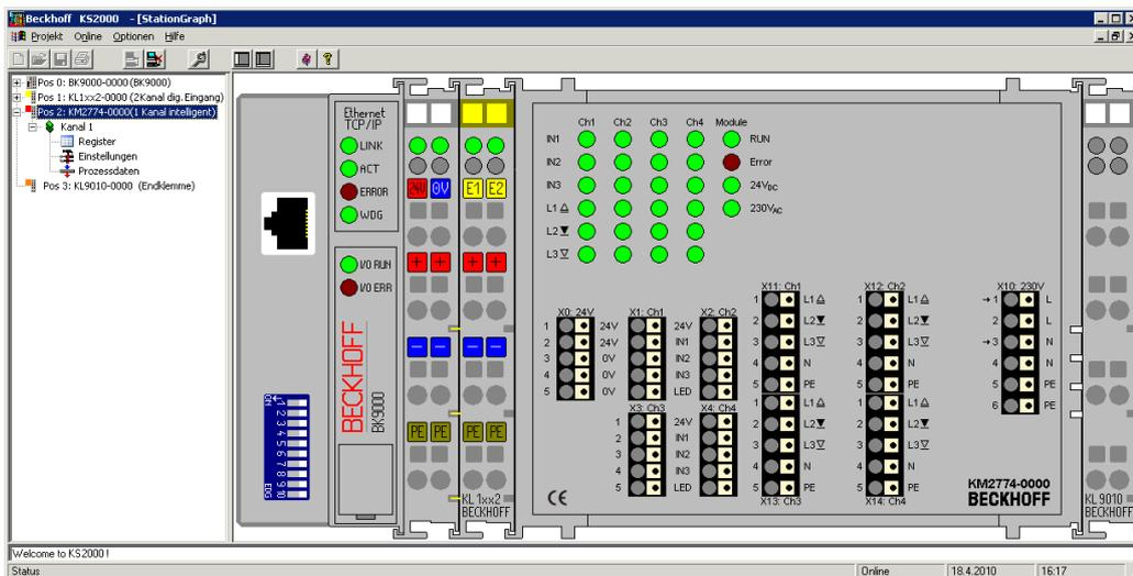
Fig. 6: Display of the fieldbus station in KS2000
