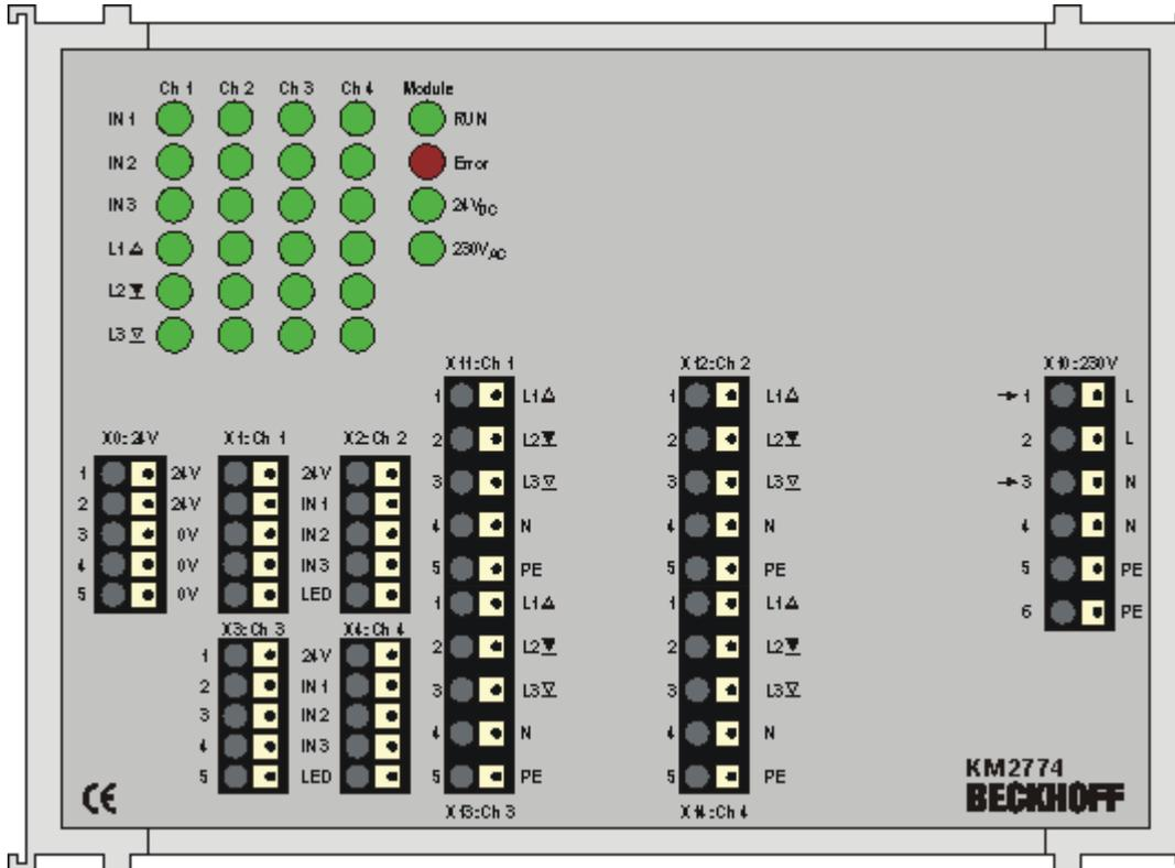
Fig. 3: KM2774 - Wiring
