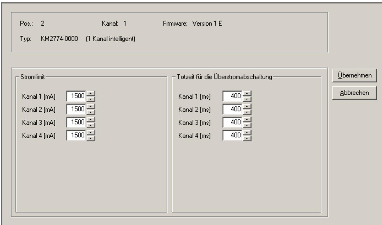
Fig. 8: Dialog screen for parameterizing the KM2774
