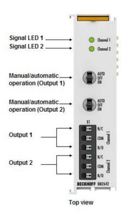
2-channel relay modules with manual and automatic operation, 230 V<sub>AC</sub>, 6 A
