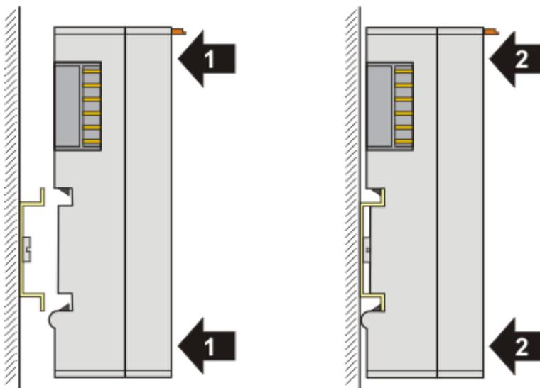
and press (1) the terminal module against the mounting rail until it latches in place on the mounting rail (2).
