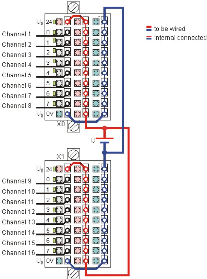
Fig. 17: Supply voltage connection
