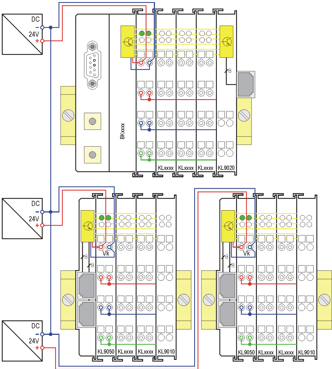
Fig. 14: KL9020, KL9050 – Connection of the power supply
