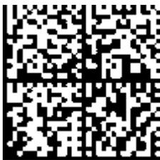
Fig. 21: Example DMC **1P**072222**S**BTNk4p562d7**1K**EL1809 **Q**1 **51S**678294
