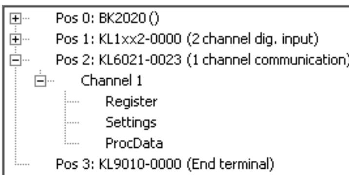
Fig. 12: KS2000 branch for channel 1 of the KL6021-0023
