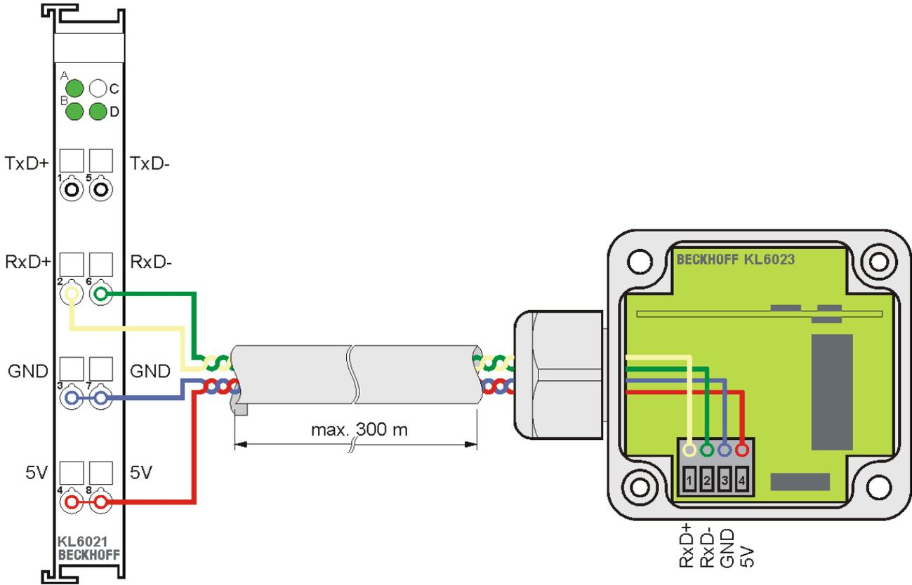
Fig. 9: Connection of the wireless adapter
