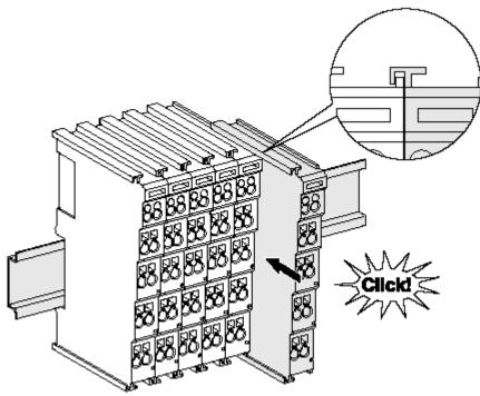
Fig. 3: Attaching on mounting rail
