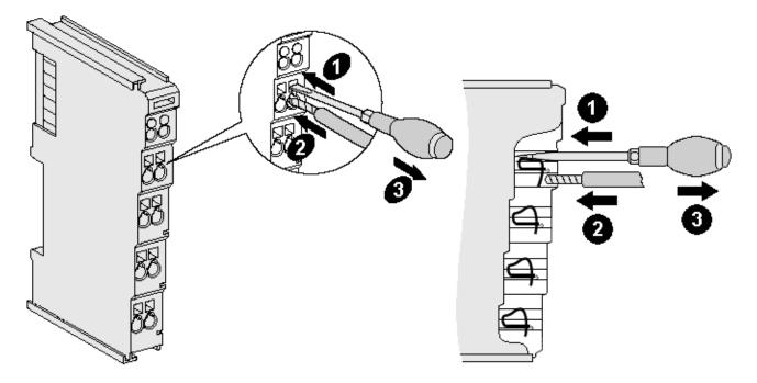
Fig. 9: Connecting a cable on a terminal point
