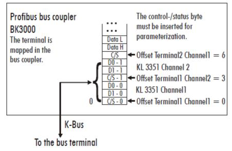
Fig. 16: Mapping in the Profibus Coupler - example for KL3351
