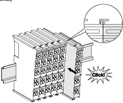
Fig. 12: Attaching on mounting rail
