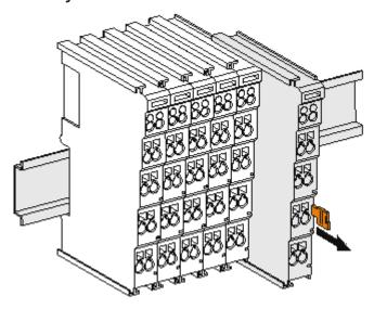
Fig. 13: Disassembling of terminal
