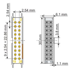
Fig. 10: Dimensions of the 20-pin contact strip in the terminal and the matching spring contact strip
