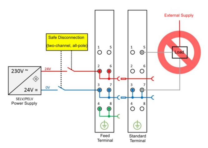
Fig. 1: Negative example – active load
