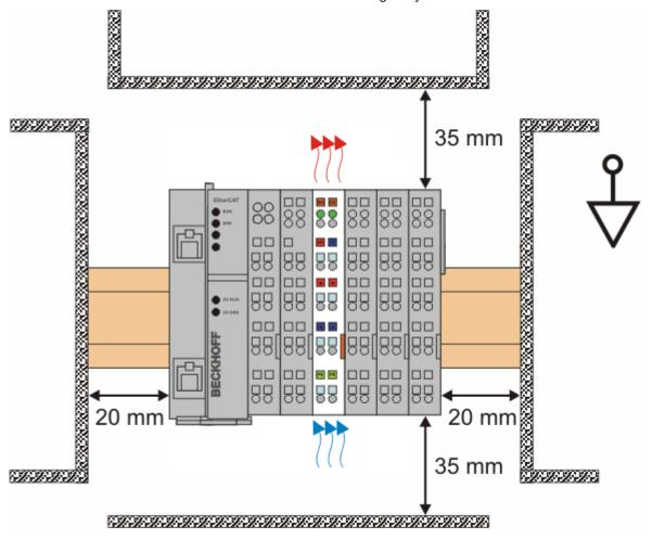
Fig. 19: Recommended distances for standard installation position
