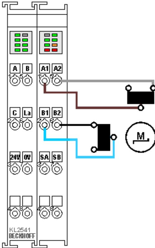
Fig. 26: KL2541 - Bipolar control of an unipolar motor
