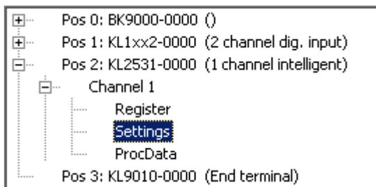
Fig. 30: KS2000 tree branches for channel 1 of the KL2531
