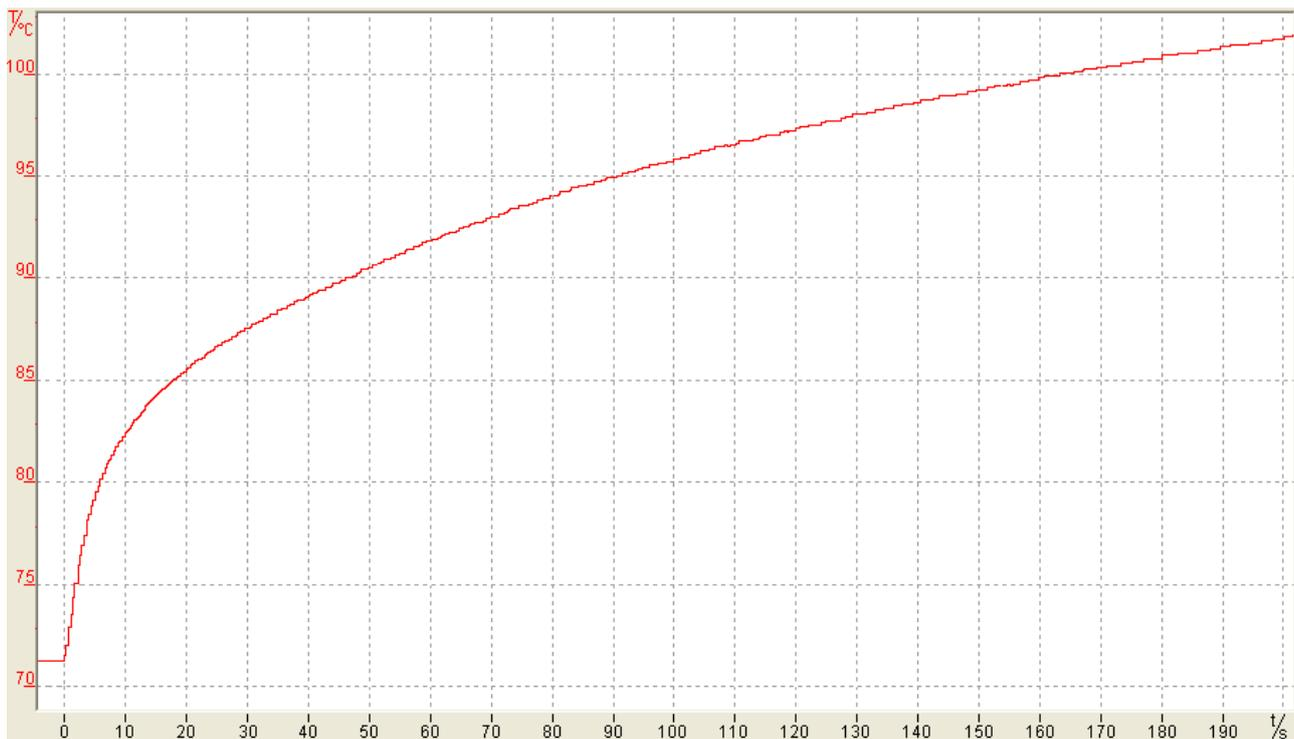
Fig. 6: KL2541 - temperature inside the housing (worst case)
