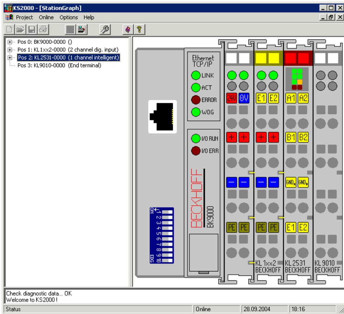
Fig. 29: Display of the fieldbus station in KS2000
