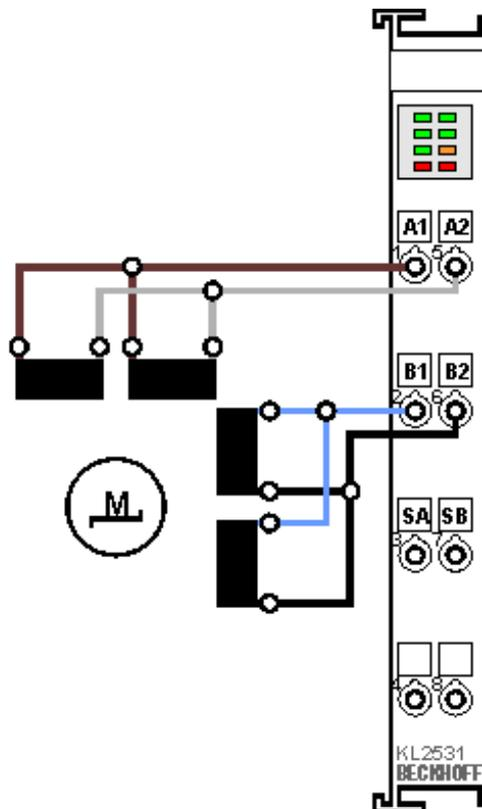
Fig. 22: KL2531 - Bipolar serial (left) and parallel (right) control of a bipolar motor
