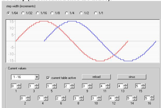
Fig. 35: KL2541 - Examples for current table settings with KS2000
