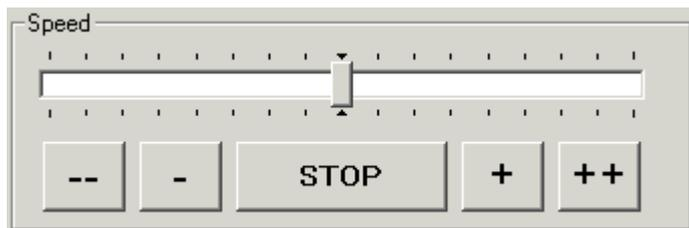
Fig. 42: Setting the velocity in the *Commissioning* tab
