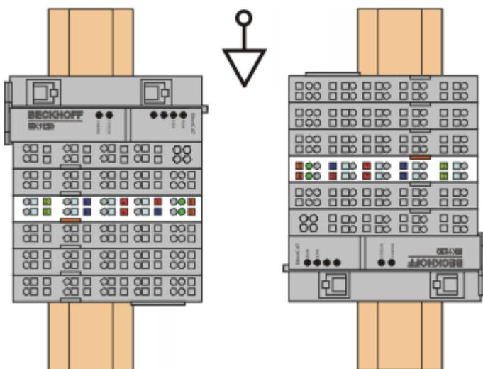
Fig. 15: Other installation positions, example 1
