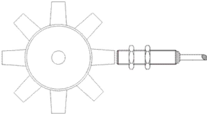
Fig. 5: Pinion with inductive proximity limit switch (register R51 = 8)
