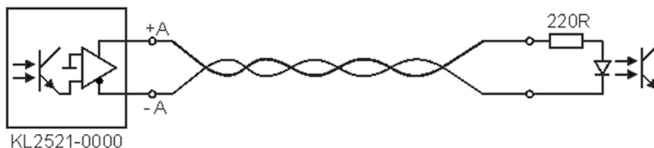
Fig. 14: EL2521-0000, direct connection to an optocoupler
