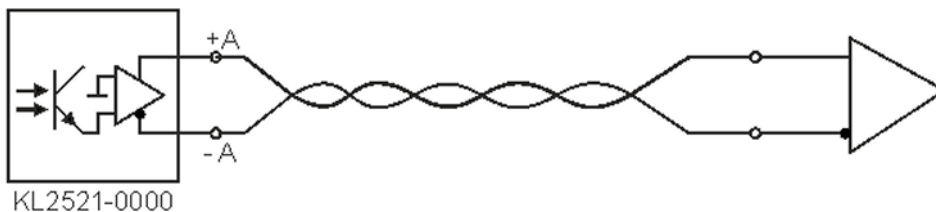
Abb. 13: KL2521-0000 am RS485/RS232 Receiver
