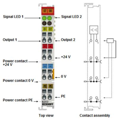
Fig. 3: KL2512 - Two-channel pulse width output terminal 24  $V_{DC}$ , ground switching
