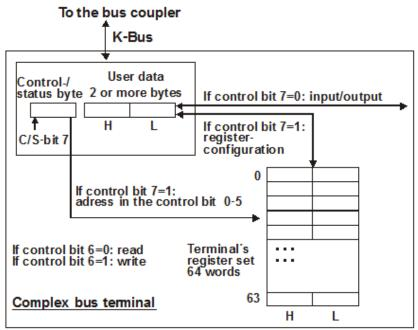
Fig. 17: Register mode control byte
