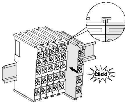
Fig. 5: Attaching on mounting rail
