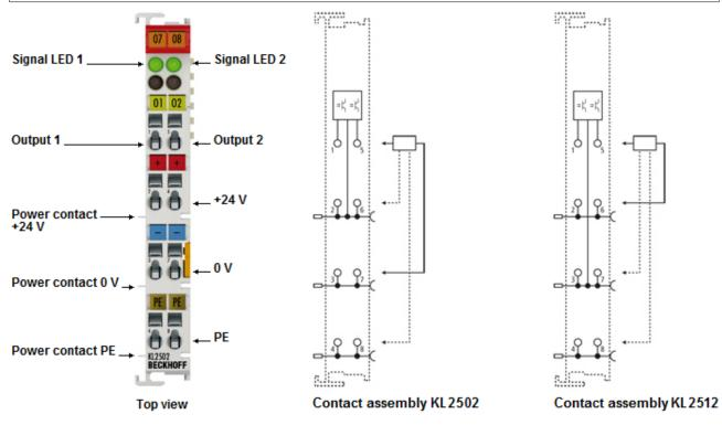
Fig. 12: KL2502, KL2512 - Contact assignment and LEDs
