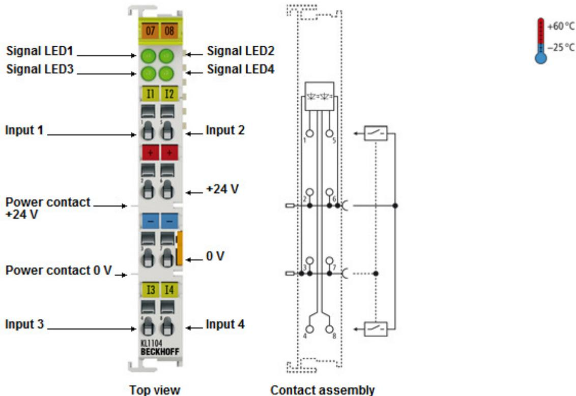
**Four channel, digital input terminals, 24 V<sub>DC</sub>**
