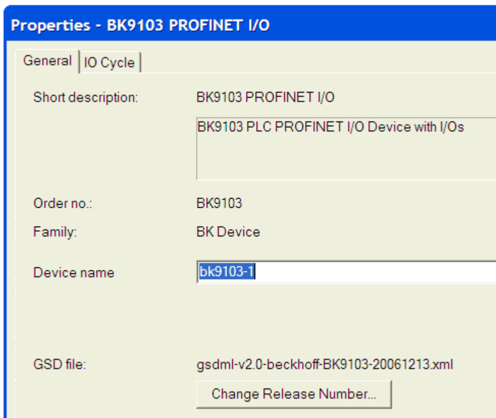
Fig. 20: Step 7 - enter the name for the PROFINET device
