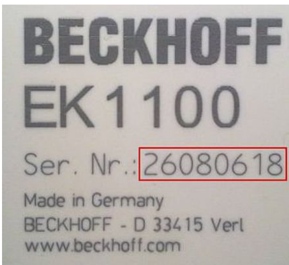
Fig. 57: EK1100 EtherCAT coupler, standard IP20 IO device with serial/ batch number
