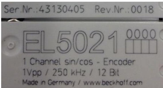
Fig. 56: EL5021 EL terminal, standard IP20 IO device with serial/ batch number and revision ID (since 2014/01)
