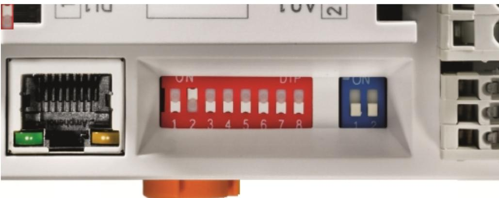
Fig. 21: Example of Ethernet IP address 172.16.21.2
