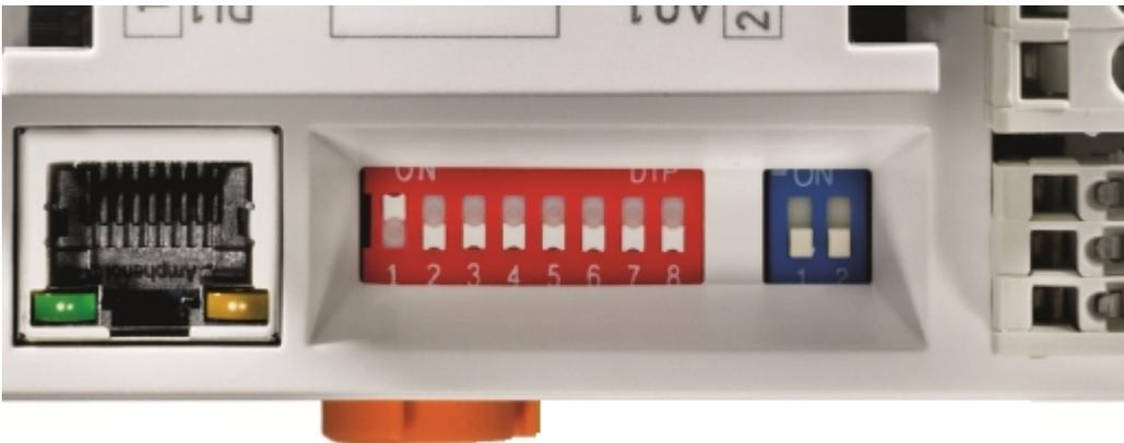
Fig. 20: Example of Ethernet IP address 172.16.21.1
