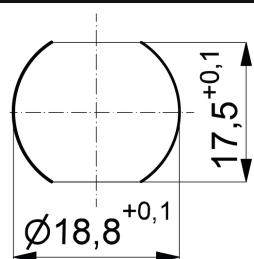
Minimum wall thickness 2,5 mm,
