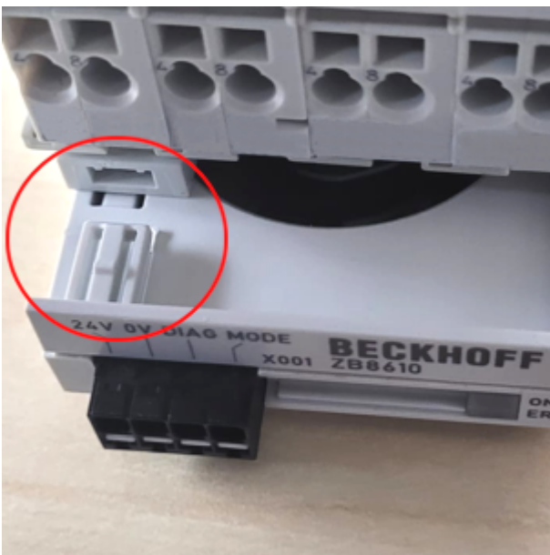
Fig. 10: Push latching tab into groove
