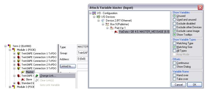
Fig. 47: Linking the variables
