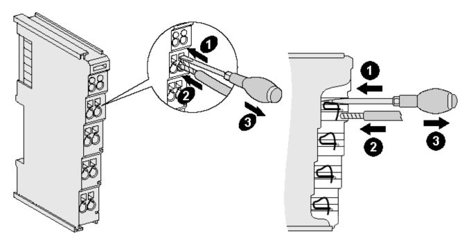
Fig. 11: Connection of a cable to a terminal point
