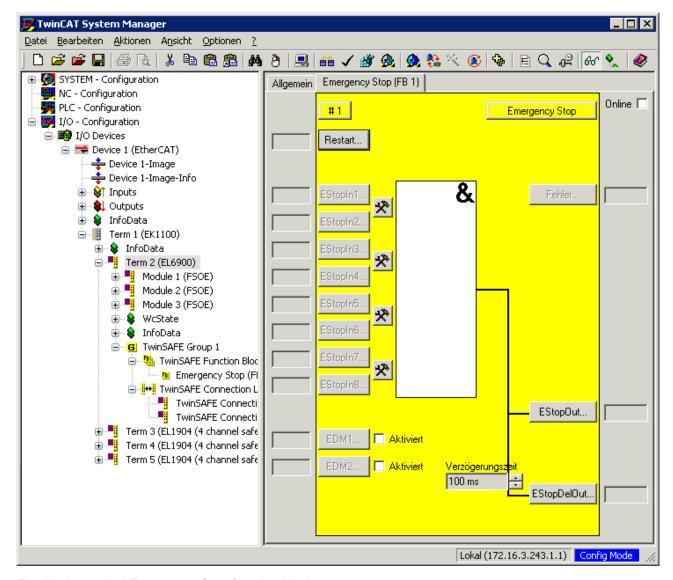
Fig. 22: Appended Emergency Stop function block
