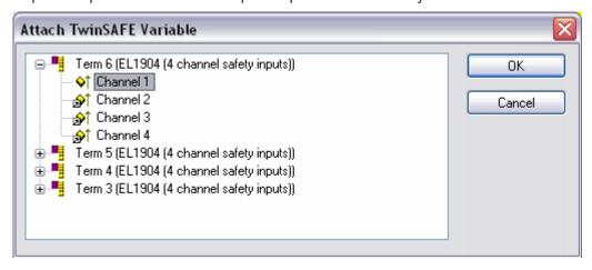
Fig. 30: Identification of inputs already in use
