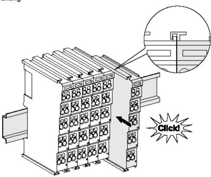
Fig. 8: Installation on the mounting rail
