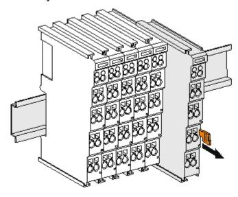
Fig. 9: Removal from mounting rail
