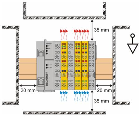
Fig. 6: Installation position and minimum distances
