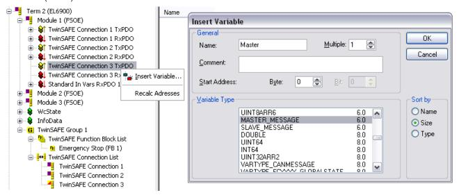
Fig. 45: Creation of a variable for the master message
