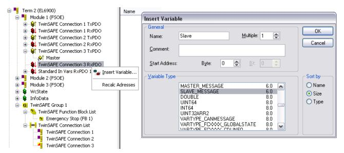
Fig. 46: Creation of a variable for the slave message
