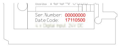
Fig. 54: Unique serial number of a TwinSAFE terminal
