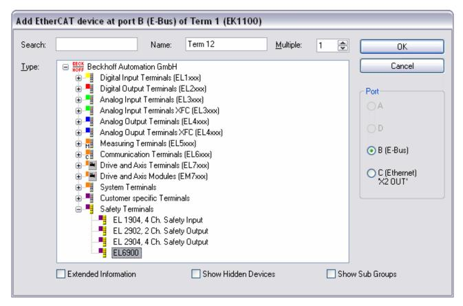
Fig. 15: Inserting an EL6900
