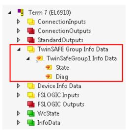
Figure 2-14: TwinSAFE group info data in the I/O tree structure
