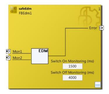
Figure 3-44: FB EDM in TwinCAT 3
