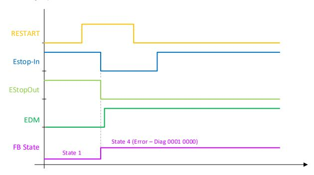
If the EDM signal of the ESTOP function block is not evaluated, the time when the change from FALSE to TRUE may occur at the Restart input is not monitored. This may also be the case before the emergency stop event. In this case the FB output is enabled when the Restart input changes from TRUE to FALSE.
