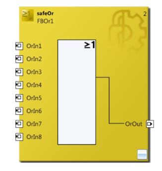
Display of the function block and its properties in TwinCAT 3.
