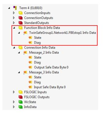
Figure 2-12: Function block info data in the I/O tree structure
