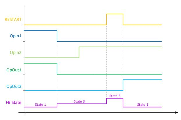
In the following diagram the Restart is set to TRUE before the operation mode change takes place. Changing the input OpIn1 from TRUE to FALSE results in a switch to state 3. Once operation mode OpIn2 is TRUE, the system changes to the Start state (FB state 6), since the Restart input is already TRUE. The output OpOut2 is activated by changing the Restart input from TRUE to FALSE.
