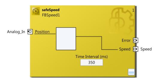
Figure 3-100: Function block SPEED
