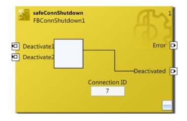
Figure 3-66: FB Connection Shutdown in TwinCAT 3
