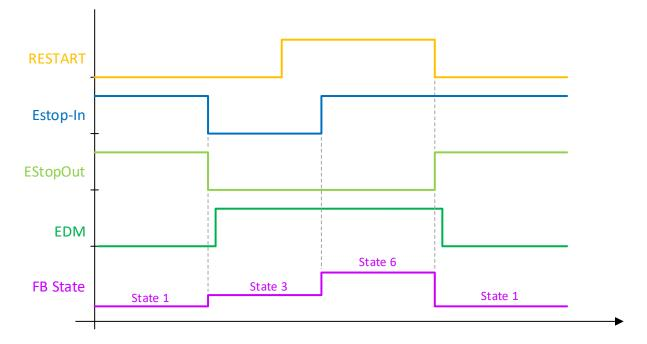
In the following diagram the Restart input is set to TRUE before the emergency stop event takes place. Due to the Restart input signal, the EDM signal is checked immediately when the EStop-In input changes from TRUE to FALSE. This immediately leads to an EDM error and to the shutdown of the entire TwinSAFE group.
