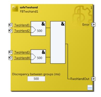
Display of the function block and its properties in TwinCAT 3.
