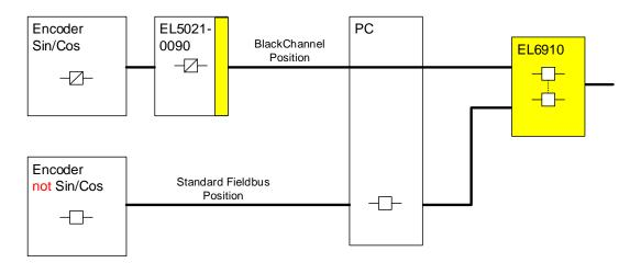
Figure 3-114: Schematic diagram of the configuration
