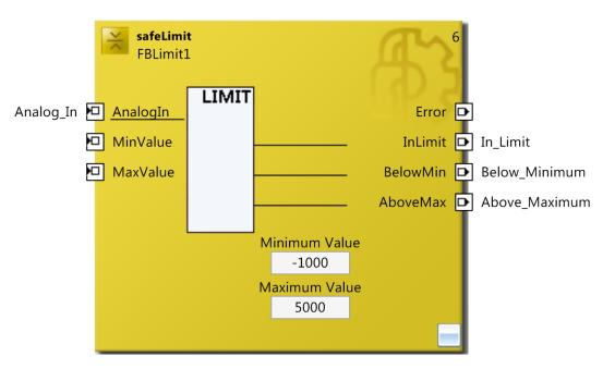
Figure 3-88: Function block LIMIT
