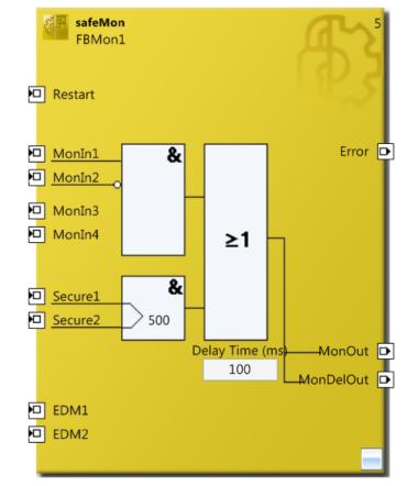
Display of the function block and its properties in TwinCAT 3.
