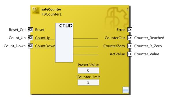
Figure 3-92: Function block COUNTER
