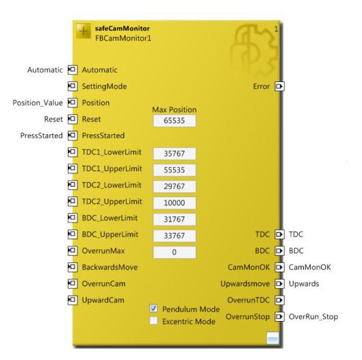
Figure 3-110: Function block CAMMONITOR
