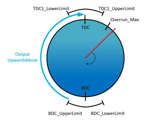
Figure 3-115: Excentric mode - schematic diagram of the ranges
