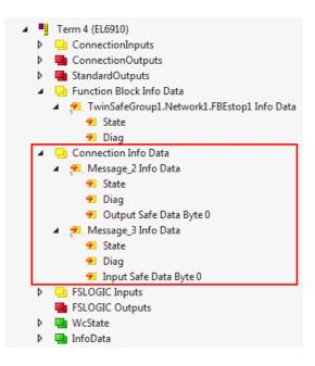
Figure 2-10: Connection info data in the I/O tree structure
