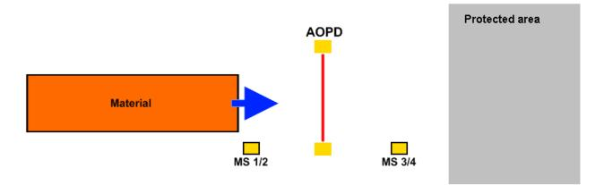
Figure 3-36: Configuration example with two two-channel muting sensors
