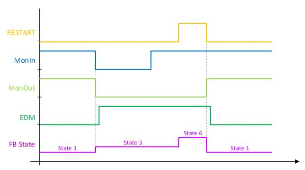
The following diagram shows the behavior of the MON function block; the rising edge of the Restart occurs before the rising edge of the MonIn inputs. The Start state (FB state 6) is only assumed if both signals are TRUE. The output is enabled with the falling edge at the Restart input. At least one of the EDM inputs of the FB is active.
