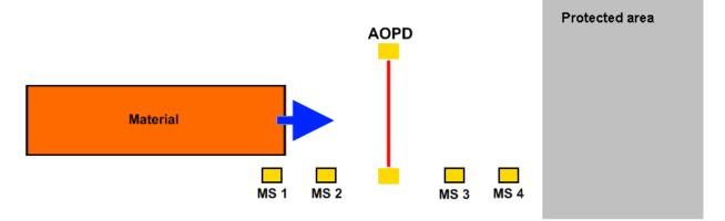
Figure 3-33: Configuration example with FB MUTING
