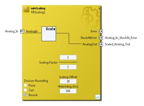
Figure 3-96: Function block SCALE
