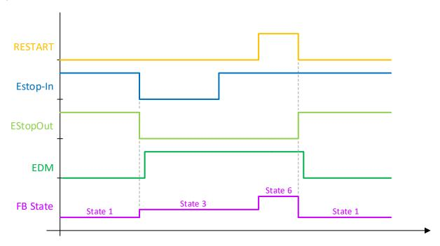
The following diagram shows the behavior of the ESTOP function block, where the change of the Restart signal from FALSE to TRUE takes place before the change of the EStop inputs from FALSE to TRUE. The Start state (FB state 6) is only assumed if both signals are TRUE. The output is enabled when the Restart input changes from TRUE to FALSE. At least one of the EDM inputs of the FB is active.
