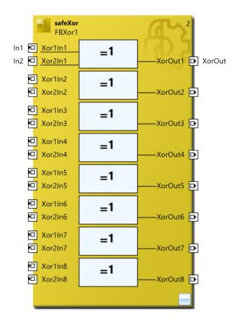
Figure 3-136: Configuration of the XOR function block
