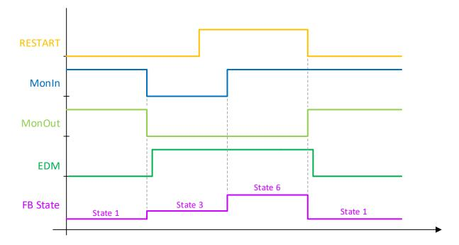
In the following diagram the Restart is set to TRUE before the MonIn event takes place. With the falling edge of the MonIn input, the EDM signal is immediately checked due to the Restart input signal. This immediately leads to an EDM error and to the shutdown of the entire TwinSAFE group. At least one of the EDM inputs of the FB is active.
