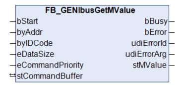
This function block reads a measured value from a GENIbus device. The operation is thereby exclusively restricted to values of class 2. Only the ID code of the high byte and the length of the measured value need to be specified; the type of scaling and the unit of the measured value are determined by an internal INFO query. A structure at the *stMValue* output provides all important information about the value.
