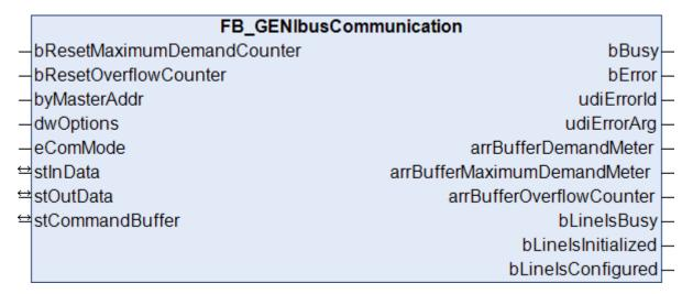
The function blocks for the GENIbus commands do not directly access the process image of the selected serial interface; instead, they place the individual GENIbus commands into three different buffers. The FB\_GENIbusCommunication() function block sequentially reads the GENIbus commands from these three
