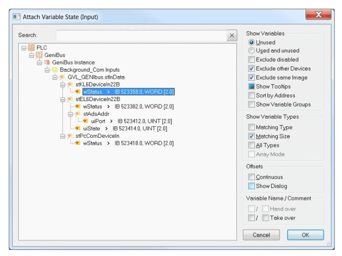
After that the data bytes can be conveniently linked to the corresponding variables by multi-link. The selection of several variables can be achieved by clicking on "Data1" and pressing the \$\psi\$ key with the Shift key pressed.
