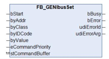
This function block writes a value in a GENIbus device or executes a command (Class-3 lds).
