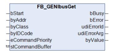
This function block reads a value from a GENIbus device.
