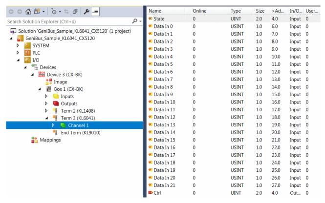
First of all, just the status is linked with the status variable of the communication input. Note that when doing so the structure for KL communication must be selected.
