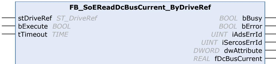
With the FB\_SoEAX5000ReadDcBusCurrent\_ByDriveRef function block the DC-Bus current (S-0-0381) can be read.
