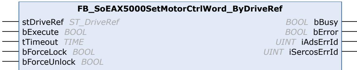
With the FB\_SoEAX5000SetMotorCtrlWord\_ByDriveRef function block the ForceLock bit (Bit 0) and the ForceUnlock bit in the Motor Control Word (P-0-0096) can be set, in order to activate or release the brake. Normally the brake is automatically controlled via the Enable of the drive.
