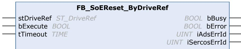
The drive (S-0-0099) can be reset with the function block FB\_SoEReset\_ByDriveRef. In the case of multiple-channel devices if necessary, both channels will have to perform a reset. The timeout time must be 10 s, as the reset can take up to 10 s depending on the error. An NC reset will not be performed.
