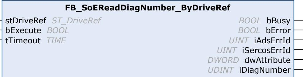
With the FB\_SoEReadDiagNumber\_ByDriveRef function block the current diagnostic number can be read as UDINT (S-0-0390).
