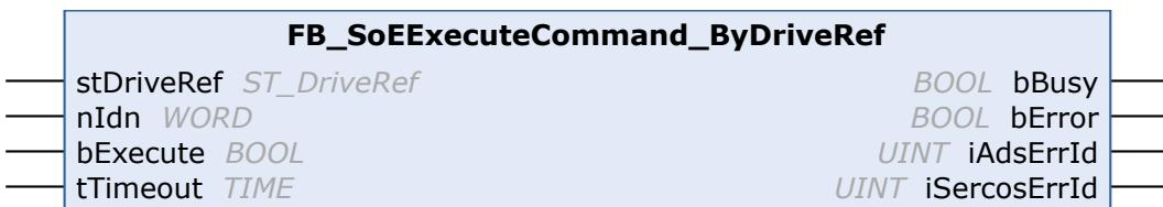
With the FB\_SoEExecuteCommand\_ByDriveRef function block a command can be executed.
