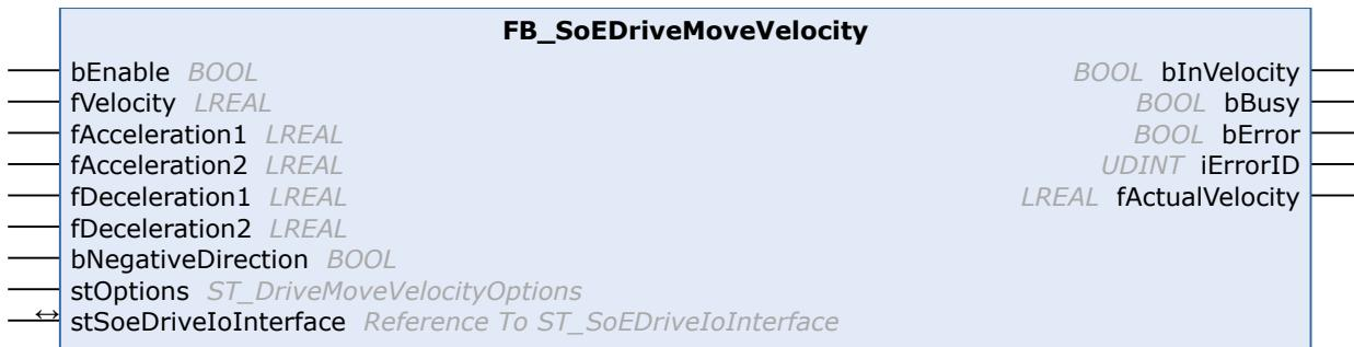
The FB\_SoEDriveMoveVelocity function block generates a simple three-phase velocity profile (without jerk limitation) that can be used to supply an SoE drive directly. Different accelerations or decelerations can be used below and above a parameterizable velocity threshold. The target velocity can be changed during operation.
