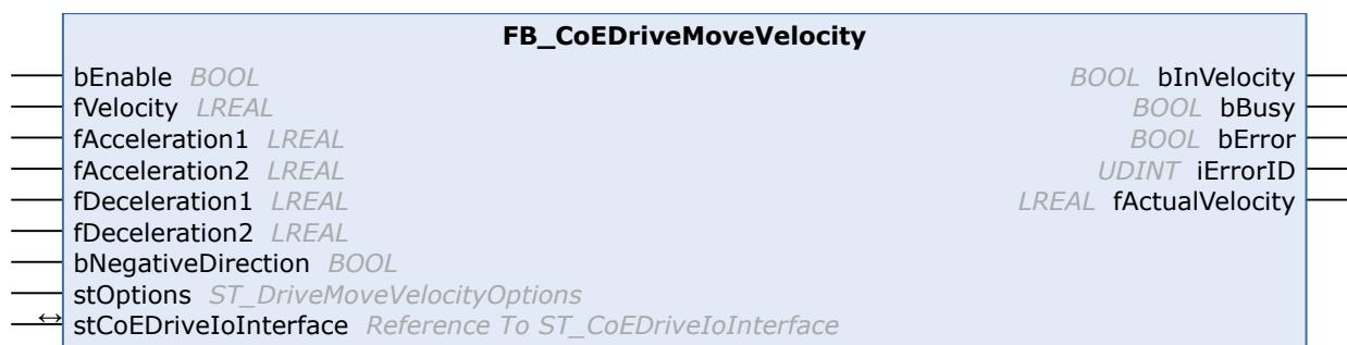
The FB\_CoEDriveMoveVelocity function block generates a simple three-phase velocity profile (without jerk limitation) that can be used to supply a CoE drive directly. Different accelerations or decelerations can be used below and above a parameterizable velocity threshold. The target velocity can be changed during operation.
