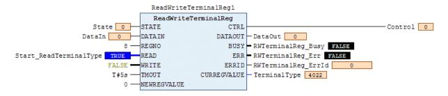
In Example 1 the terminal identifier is read from register 8 of an analog output terminal. The variables *State*, *Control*, *DataIn* and *DataOut* are linked to the terminal's corresponding I/O variables in the TwinCAT System Manager. The terminal identifier is KL**4022**..
