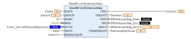
In Example 2 the user-scaling is activated in the feature register (register 32) of a KL4022 analog output terminal. The new value in the feature register is then read by the function block, and can be checked through the output variable **CURREGVALUE**.
