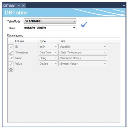
The specific table type offers the option to distribute the individual symbols that were set in the symbol group to the table columns in the database as required. When a data set is written to the database in AutoLog mode, the current values of the symbol group at the sampling time are saved in the corresponding table column.
