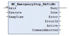
The function block cancels a current axis motion and monitors the emergency stop operation.
