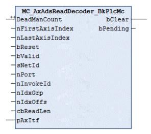
The function block decodes ADS read accesses. The <u>ADS codes [) 337]</u> are listed in the Knowledge Base.
