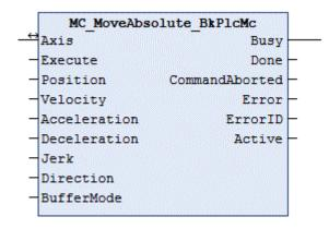
This function block starts and monitors the movement of an axis.
