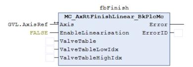
If the use of the characteristic curve is not enabled or not possible, an internal function block is used for sectional linearization. This is the case if at least one of the following reasons applies:
