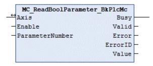
This function block reads the boolean parameters of an axis. The function block <u>MC ReadParameter BkPlcMc</u> [ $\blacktriangleright$  <u>35]</u> is available for non-boolean parameters.
