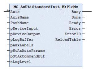
The function block handles the initialization and monitoring of axis components.
