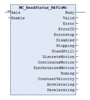
The function block determines the current state of an axis.
