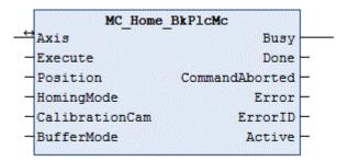
This function block starts and monitors the homing of an axis.
