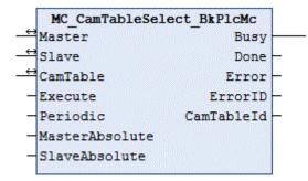
The function block initializes a variable of type <u>MC\_CAM\_ID\_BkPlcMc [> 119]</u>, thereby preparing a cam plate for the coupling of two axes.
