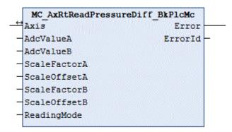
The function block handles determination of the actual pressure of the axis from the input data of two analog input terminals.
