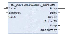
The function block automatic determines a number of axis parameters.
