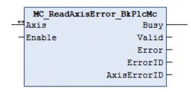
This function block determines the current error code of an axis.
