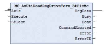
The function block reads the contents of a register from the KL terminal, which is used as drive interface for the axis.
