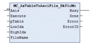
The function block writes the contents of a table to a text file.
