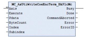
The function block writes the contents of a register of the EL terminal, which is used as encoder interface for the axis.
