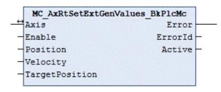
The function block supplies an axis with command variables, which do not originate from the axis' own generator.
