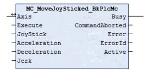
This function block starts and monitors the movement of an axis.
