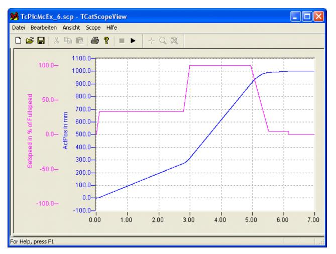
This profile is created on restart in the same direction with a different velocity (higher in this case).
