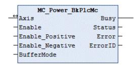
The function block is used to control an external actuator. Further information on this topic can be found under <u>FAQ #9 [ $\triangleright$  321].</u>
