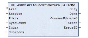
The function block writes the contents of a register of the EL terminal, which is used as drive interface for the axis.
