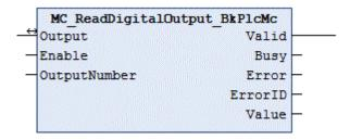
The function block determines the current state of a digital output of a cam controller.
