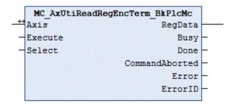
The function block reads the contents of a register from the KL terminal, which is used as encoder interface for the axis.
