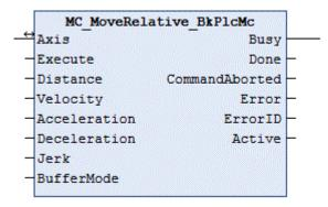
This function block starts and monitors the movement of an axis.
