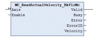
The function block determines the current velocity of an axis.
