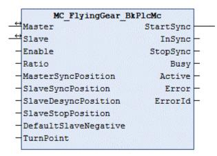
The function block takes over the control of a flying gear coupling.
