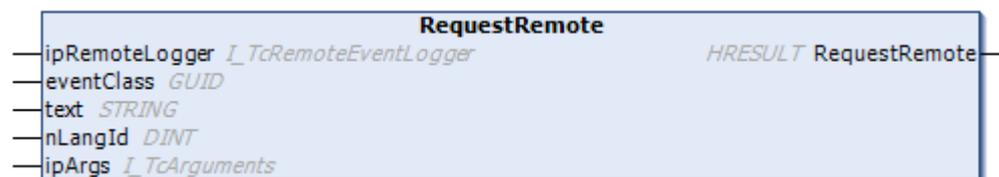
Calling this method triggers the asynchronous request on a remote target system.
