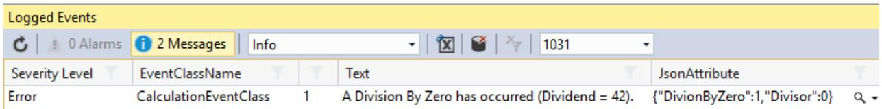
The Logged Events window provides two visualizations for the JSON attributes, which can be selected via the drop-down menu inside the information column and opened by clicking on the magnifying glass:
