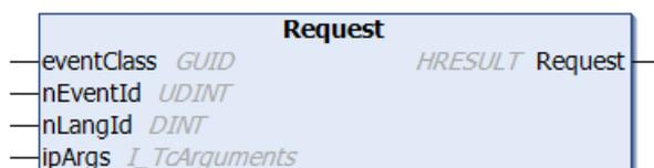
Calling this method triggers the asynchronous text request.
