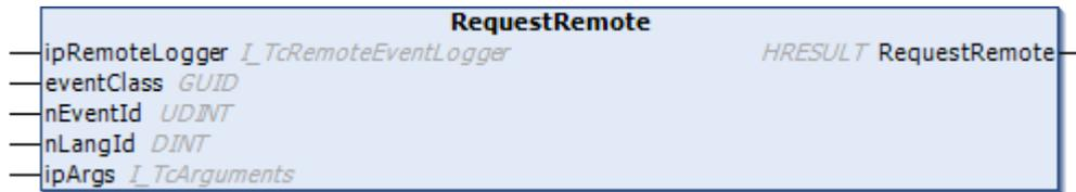
Calling this method triggers the asynchronous request on a remote target system.
