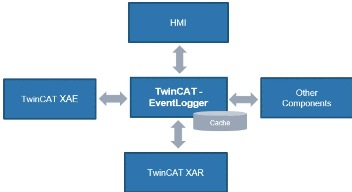
The TwinCAT 3 EventLogger keeps a limited number of the last events in a cache. This can be queried from the Engineering, for example after a restart, in order to enable a diagnosis to be made. The cache is dependent on the secured shutdown of the computer.
