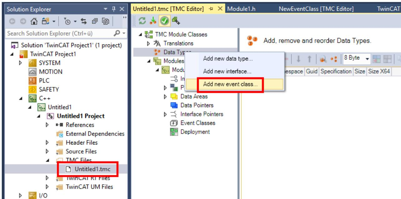
The event classes are declared for use in the corresponding C++ modules (irrespective of where they were defined). If an event class is added to a C++ module, it is automatically embedded in the TMC file of the module.
