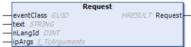
Calling this method triggers the asynchronous text request.
