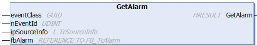
This method returns an interface pointer to an existing instance.
