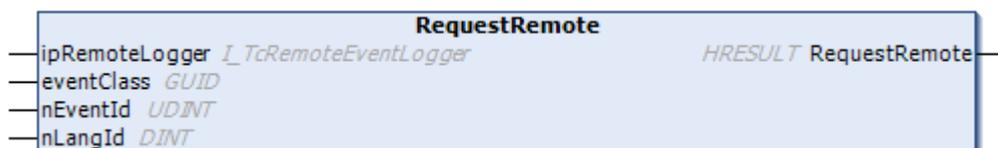
Calling this method triggers the asynchronous request on a remote target system.
