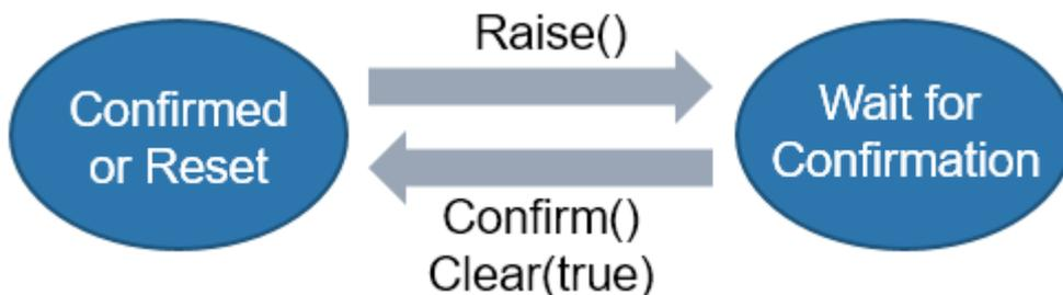
Calling the corresponding methods causes an event to be transmitted and sets the alarm to the respective state.
