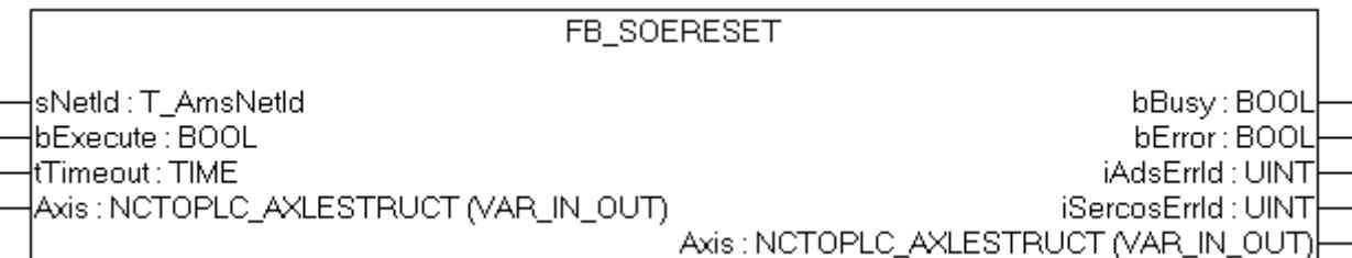
The functionblock FB\_SoEReset can be used to execute a drive reset (S-0-0099). Drives with more than one channel may require a reset on all channels. The timeout time must be 10s, because the reset can take up to 10s.
