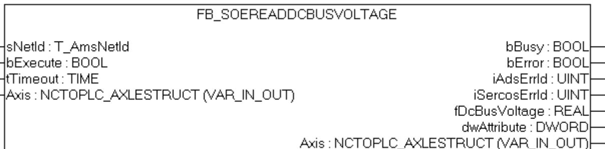
The functionblock FB\_SoEReadDcBusVoltage can be used to read the DC-Bus-Voltage of the amplifier (S-0-0380).
