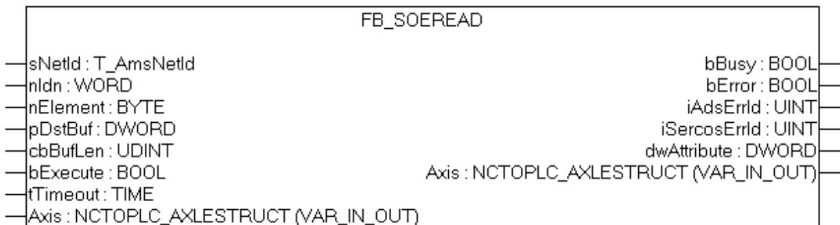
The functionblock `FB_SoERead` can be used to read a parameter.
