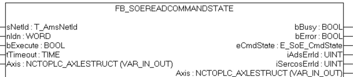
The function block FB\_SoEReadCommandState can be used to read the state of a command.
