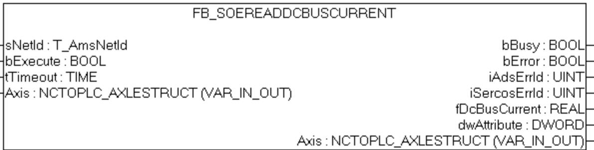
The functionblock FB\_SoEAX5000ReadDcBusCurrent\_ByDriveRef can be used to read the DC-Bus-Current (S-0-0381).
