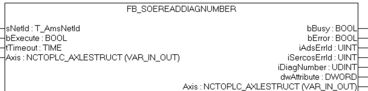
The functionblock FB\_SoEReadDiagNumber can be used to read the actual diagnose number as UDINT (S-0-0390).
