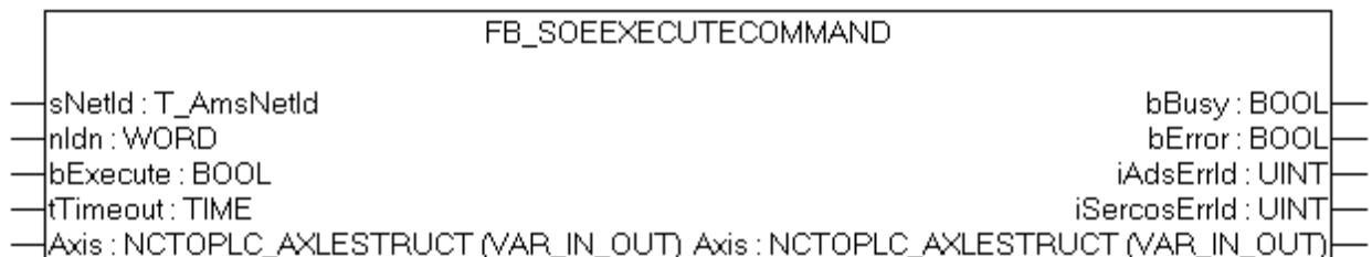
The functionblock FB\_SoEExecuteCommand can be used to execute a command.
