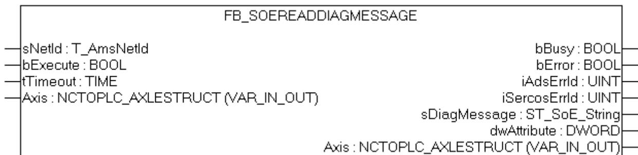
The functionblock FB\_SoEReadDiagMessage can be used to read the diagnose message as a Sercos-String (S-0-0095).
