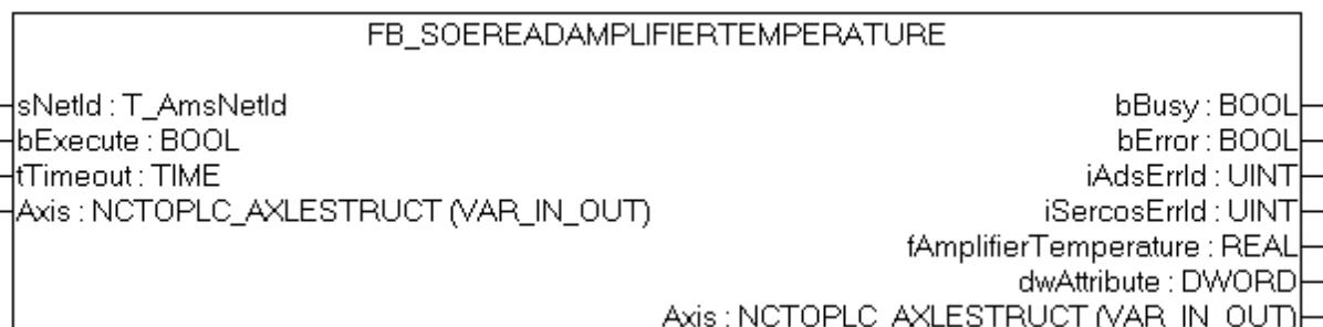
The functionblock FB\_SoEReadAmplifierTemperature can be used to read the amplifier temperature (S-0-0384).
