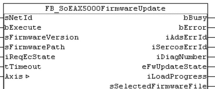
The functionblock FB\_SoEAX5000FirmwareUpdate can be used to check and update the firmware of the AX5000 to a requested version (revision and build) or to the newest build of the configured revision.
