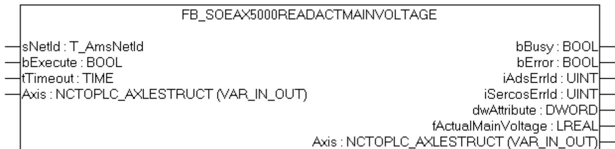
The functionblock FB\_SoEAX5000ReadActMainVoltage can be used to read the main voltage (P-0-0200) of the AX5000.
