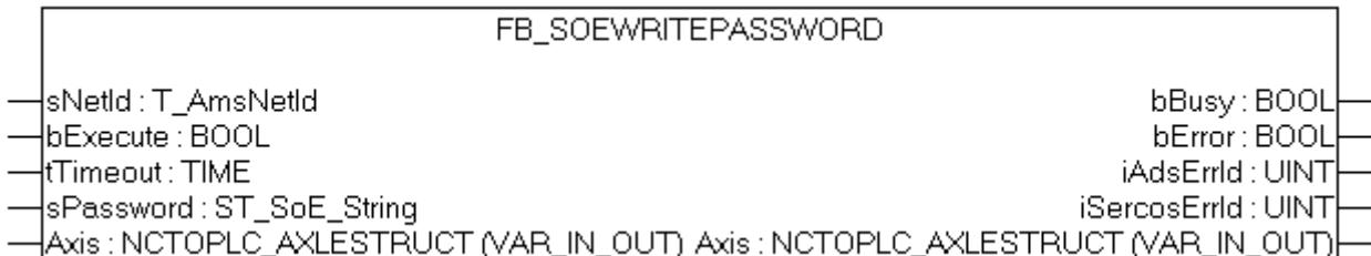
The functionblock FB\_SoEWritePassword can be used to set the drive password (S-0-0267).
