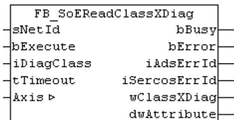
The function block FB\_SoEReadClassXDiag can be used to read the actual Class 1 Diagnose (S-0-0011) ... Class 3 Diagnose (S-0-0013) as a WORD. There is a conversion function F\_ConvWordToSTAX5000C1D for evaluation of the Class 1 Diagnose as a structure ST\_AX5000\_C1D. See Documentation of TcDrive.lib.
