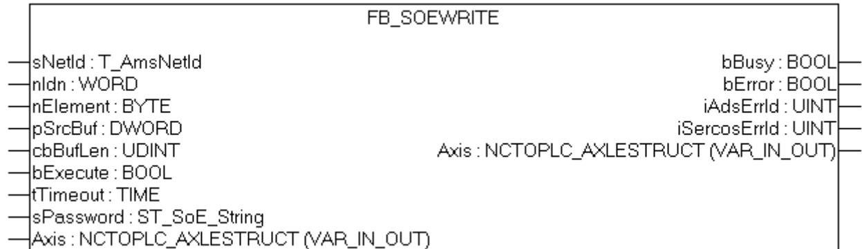
The functionblock FB\_SoEWrite can be used to write a parameter.
