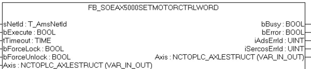
The functionblock FB\_SoEAX5000SetMotorCtrlWord can be used to set the ForceLock-Bit (Bit 0) or the ForceUnlock-Bit in the motor control word (P-0-0096), in order to set or release the brake. The brake is set and released automatically via the enable of the drive.
