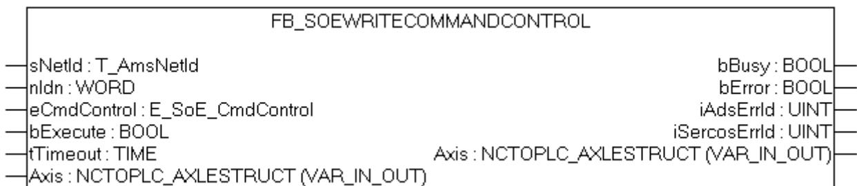
The functionblock FB\_SoEWriteCommandControl can be used to prepare, start or cancel a command.
