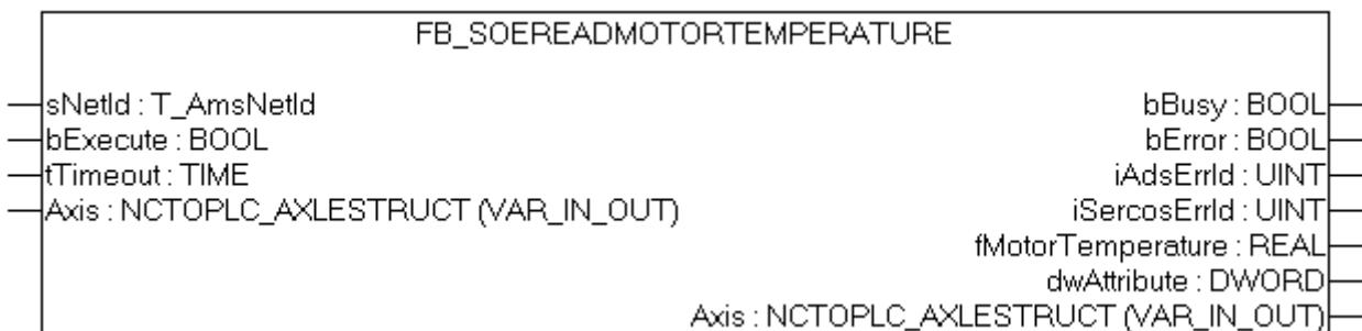
The functionblock FB\_SoEReadMotorTemperature can be used to read the temperature of the motor (S-0-0383). If the motor does not contain a temperature sensor then the FB reports 0.0, means 0.0°C.
