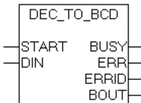
The "DEC\_TO\_BCD" function block allows decimal numbers to be converted to BCD format. The number to be converted is checked for admissibility of the values.
