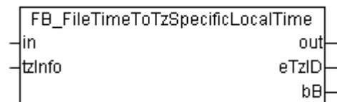
The function block converts the UTC time (file time format) to local time (file time format), taking into account the specified time zone information. The function block [FB\\_SystemTimeToTzSpecificLocalTime \[▶ 189\]](#) has similar functionality but uses a different time format (structured system time format).
