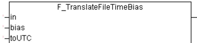
This function converts the input time to the time in another time zone based on the specified bias time shift. The function can be used to convert the local time to UTC time (Universal Time Coordinates) and vice versa, for example.
