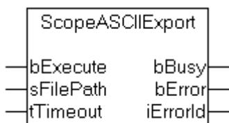
The function block "ScopeASCIIExport" allows the Scope View to be exported into an ASCII file. Currently this function can only be used if only one view (such as Scope View 1) is active in the application. Internally, an instance of the ADSWRITE function block is called.
