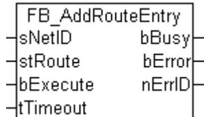
This function block adds a new AMS Router connection (remote route) to a TwinCAT System.
