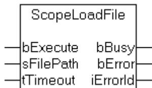
The function block "ScopeLoadFile" allows a Scope View Configuration Project (\*.scp) to be loaded into the TwinCAT Scope View. Internally, an instance of the ADSWRITE function block is called.
