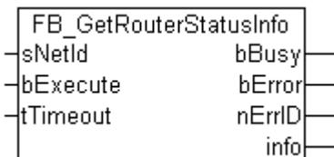
The function block FB\_GetRouterStatusInfo reads the TwinCAT Router status information (available memory, number of registered ports... ).
