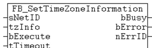
This function block can be used to modify or set the time zone settings of the operating system.
