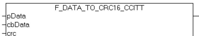
The function "F\_DATA\_TO\_CRC16\_CCITT" performs a 16-Bit-CRC-CCITT (cyclic redundancy check) of any data. Internally the function [F\\_BYTETO\\_CRC16\\_CCITT \[▶ 54\]](#) is used, refer to the documentation of the [F\\_BYTETO\\_CRC16\\_CCITT \[▶ 54\]](#) function for further information.
