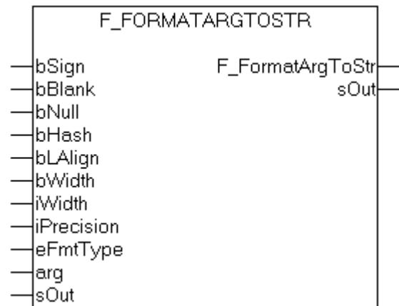
Auxiliary format function. This function is used internally by the FB\_FormatString [▶ 157] function block. The function can be used to convert a variable of type T\_Arg [▶ 239] into a formatted string according to the format specification [▶ 274].
