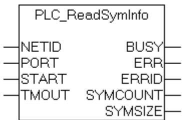
The "PLC\_ReadSymInfo" function block permits information regarding the symbols (variables) of a PLC run-time system. Internally, an instance of the ADSREAD function block is called.
