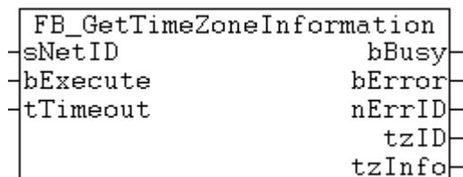
With this function block the time zone settings of the operating system can be read.
