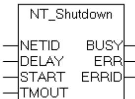
The Windows NT operating system can be shut down with the aid of the "NT\_Shutdown" function block. The function largely corresponds to the Shut Down command on the Windows taskbar. A delay before execution of the Shut Down command can be defined via the DELAY parameter. Internally, an instance of the ADSWRTCTRL function block is called.
