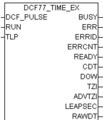
The "DCF77\_TIME\_EX" function block can be used to decode the DCF-77 radio clock signal. In contrast to the [DCF77\\_TIME \[▶ 221\]](#) function block, this block checks two consecutive telegrams for plausibility as standard.
