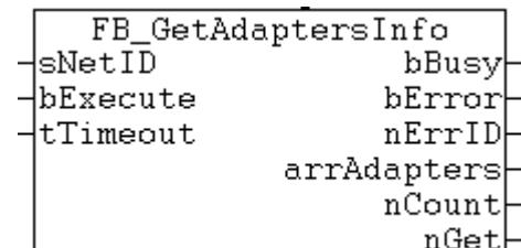
The function block retrieves adapter information for the local or remote TwinCAT computer. The max. number of read adapter information is limited to MAX\_LOCAL\_ADAPTERS + 1 (default = 6).
