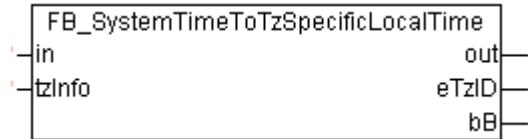
The function block converts the UTC time (structured system time format) to local time (structured system time format), taking into account the specified time zone information. The function block
