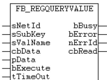
The System registration is a hierarchical structured tree. A node in the tree is called key. Each Key again can contain SubKeys, and Values.
