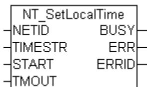
The function block "NT\_SetLocalTime" sets the local Windows system time of the TwinCAT system (the local Windows system time is displayed in the task bar).
