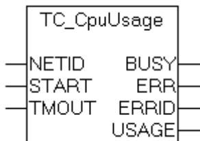
The "TC\_CpuUsage" function block allows the current CPU loading of a TwinCAT system to be determined. This function corresponds to the display of CPU loading in the TwinCAT system menu under the real-time settings. Internally, an instance of the ADSREAD function block is called.
