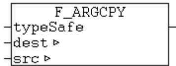
This function copies the value of a variable of type T\_Arg into another variable and supplies the number of successfull copied databytes as return value.
