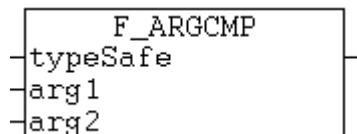
This function compares two variables of type T\_Arg and supplies the result as return parameter.
