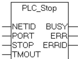
The function block "PLC\_Stop" can be used to stop a PLC run-time system on a TwinCAT computer. The function block can, for instance, be used to stop the PLC on a remote or a local PC. Internally, an instance of the ADSWRTCTRL function block is called.
