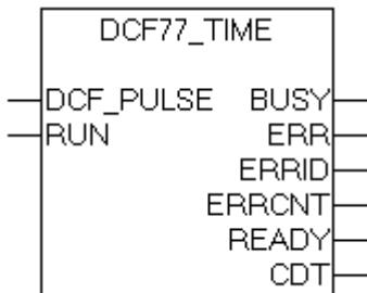
The "DCF77\_TIME" function block can be used to decode the DCF-77 radio clock signal.
