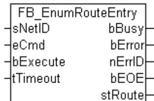
This function block is used to transfer information to other TwinCAT systems via the AMS router connections (remote routes). If several connections are used the function block must be called up repeatedly. Only one entry can be handled for each call. The input parameter *eCmd* is used for navigating through the list of entries. The *eCmd* input determines whether the first or the next input is read.
