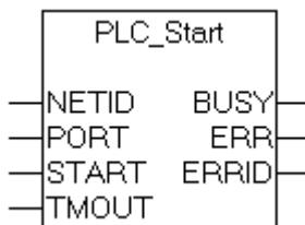
The function block "PLC\_Start" can be used to start a PLC run-time system on a TwinCAT computer. The function block can, for instance, be used to start the PLC on a remote PC.
