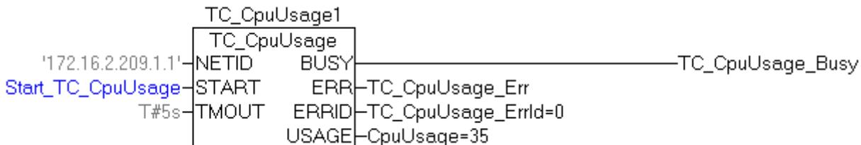
In the example the TwinCAT system is using 35% of the total available CPU computing time.
