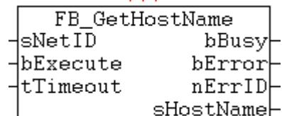
This function block reads the local host name of the TwinCAT computer.
