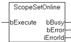
The function block "ScopeSetOnline" places the Scope View into the online state. Internally, an instance of the ADSWRITE function block is called.
