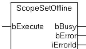
The function block "ScopeSetOffline" places the Scope View into the offline state. Internally, an instance of the ADSWRITE function block is called.
