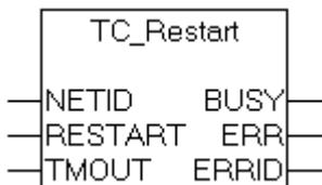
The function block "TC\_Restart" can be used to restart the TwinCAT system. The function corresponds to the Restart command on the TwinCAT system menu (on the right of the Windows taskbar). Restarting the TwinCAT system involves the TwinCAT system first being stopped, and then immediately started again. Internally, an instance of the ADSWRTCTRL function block is called.
