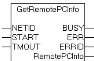
The function block "GetRemotePCInfo" permits information about configured remote PCs in the TwinCAT Router to be read. After successful execution, the structure "RemotePCInfo" contains the NetIds and names of the remote PCs as strings, in the same sequence as that in which they are stored in the TwinCAT Router. Internally, an instance of the ADSREAD function block is called. The function block allows router information relating to either a local or to a remote TwinCAT system to be read.
