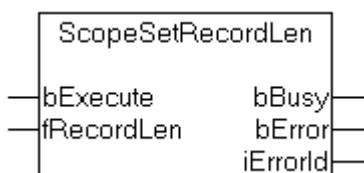
The function block "ScopeSetRecordLen" can be used to configure the Scope View recording time. Currently this function can only be used if only one view (such as Scope View 1) is active in the application. Internally, an instance of the ADSWRITE function block is called.
