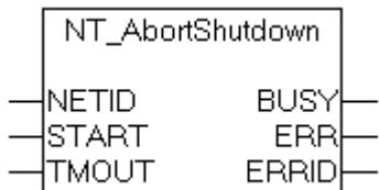
The "NT\_AbortShutdown" function block can be used to abort a shutdown command that has previously been called with the NT\_Shutdown [▶ 126] function block. Internally, an instance of the ADSWRTCTRL function block is called.
