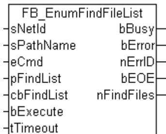
This function block searches a directory for a file or a subdirectory whose name is similar to the specified name. Any entries found can be read individually. See also description of the [FB\\_ElemFindFileEntry \[▶ 158\]](#) function block. The input parameter **eCmd** is used for navigating through the list of entries. The **eCmd** input determines whether the first or the next input is read, for example.
