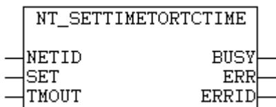
The function block "NT\_SetTimeToRTCTime" can be used to synchronise the local Windows system time (displayed in the task bar) with the real-time clock of the PC (RTC time in the BIOS).
