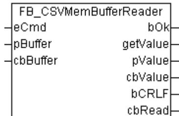
This function block can be used to decompose/interpret data sets stored in an external buffer into individual data fields. The buffer data could first be read from a file with the aid of the function blocks for file access, for example. The function block reads the first or the next data field and returns its value either as a string at the *getValue* output or as an address/byte value at the *pValue/cbValue* output.
