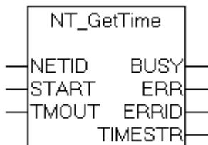
The local Windows system time of a TwinCAT system can be obtained using the "NT\_GetTime" function block (the local Windows system time is displayed in the task bar). The year, month, day, day of the week, hour, minute, second and millisecond are placed in the variables in the structure TIMESTRUCT [▶ 230]. Internally, an instance of the ADSREAD function block is called.
