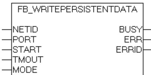
The function block FB\_WritePersistentData is an extended version of [WritePersistentData \[▶ 216\]](#) function block. The input parameter MODE affects the system behaviour of how the persistent data is written. For additional info see: [Writing of persistent data: System behaviour \[▶ 276\]](#).
