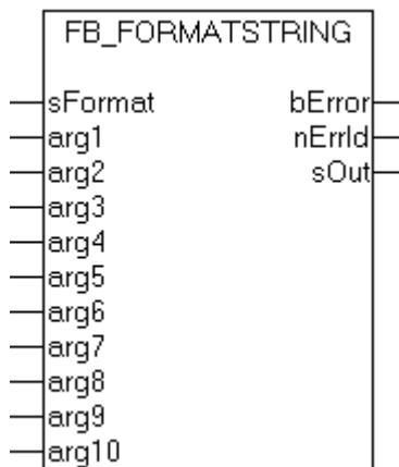
This function block can be used for converting up to 10 arguments (similar to `fprintf`) into a string and formatting them according to the [format specification \[▶ 274\]](#). Formatting occurs in the same PLC cycle, i.e. the output string is available immediately after the FB was called.
