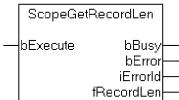
The function block "ScopeGetRecordLen" allows the recording time for the Scope View that is currently configured in TwinCAT Scope View to be determined. Currently this function can only be used if only one view (such as Scope View 1) is active in the application. Internally, an instance of the ADSREAD function block is called.
