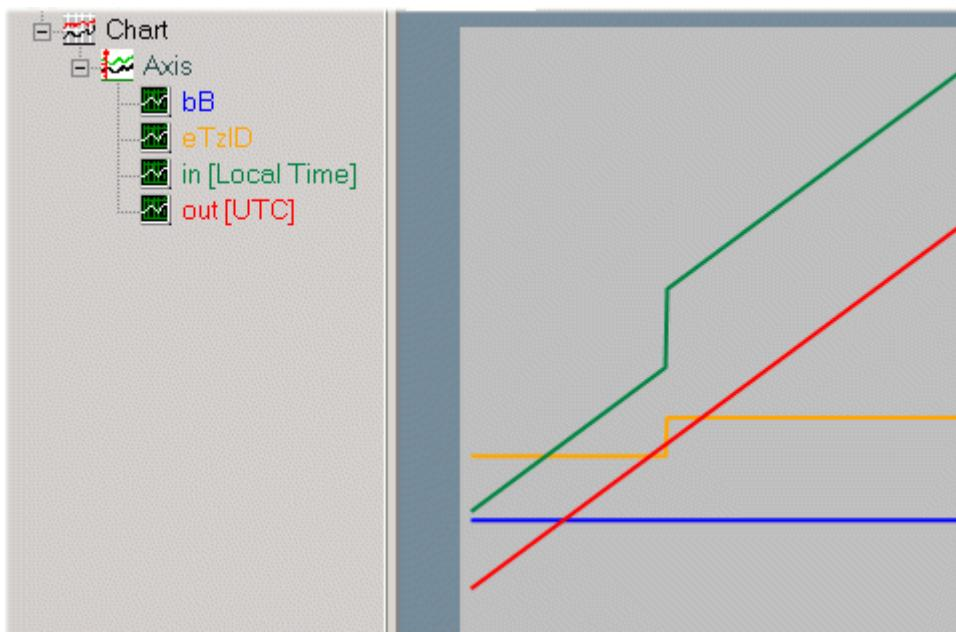
The local time (green) jumps forward. The UTC output time (red) continuous. The local time: **2h:59m:59s:999ms..** is directly followed by: **3h:00m:00s:000ms..**. The time zone ID (orange) changes from *eTimeZoneID\_Standard* (standard time) to *eTimeZoneID\_Daylight* (daylight-saving time).
