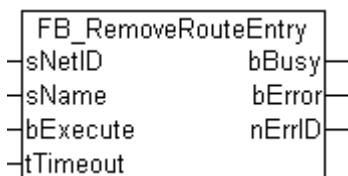
This function block deletes an existing connection to a TwinCAT System from the AMS Router Connection (remote routes) list.
