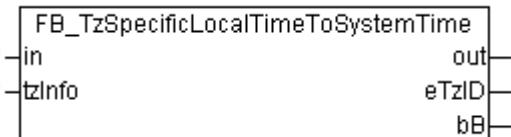
The function block converts the local time (structured system time format) to UTC time (structured system time format), taking into account the specified time zone information. The function block
