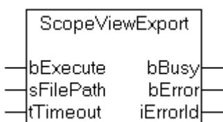
The function block "ScopeViewExport" allows a Scope View to be exported into a file (\*.svw). Currently this function can only be used if only one view (such as Scope View 1) is active in the application. Internally, an instance of the ADSWRITE function block is called.
