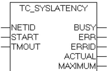
The "TC\_SysLatency" function block allows the current and maximum latency time of a TwinCAT system to be determined. This function corresponds to the display of latency time in the TwinCAT system menu under the real-time settings. Internally, an instance of the ADSREAD function block is called.
