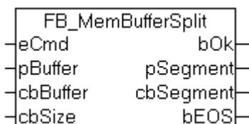
This function block splits a memory area (data buffer) into several smaller segments of certain maximum length as required. The function block returns a smaller partial segment, if the length of the last segment is smaller than required.
