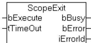
The function block "ScopeExit" terminates one instance of TwinCAT Scope View. Internally, an instance of the ADSWRITE function block is called.
