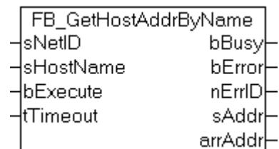
The function block reads hosts (IPv4) Internet Protocol network address corresponding to a host name from a host database. The address is returned as string and byte array.
