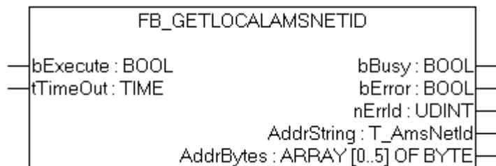
The function block FB\_GetLocalAmsNetId reads the local AmsNetId (local TwinCAT-specific network address).
