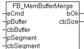
This function block consolidates individual smaller data segments to form a larger data segment. The target buffer must be transferred as input parameter to the block. No further data bytes are added, if the segment to be added exceeds the remaining free buffer size.
