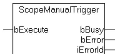
The Scope View can be triggered manually with the function block "ScopeManualTrigger". Currently this function can only be used if only one view (such as Scope View 1) is active in the application. Internally, an instance of the ADSWRITE function block is called.
