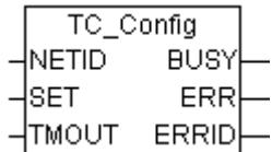
A TwinCAT system in RUN mode (green TwinCAT system icon) can be switched to CONFIG mode (blue TwinCAT system icon) via the function block "TC\_Config". If the system is already in CONFIG mode, it is first switched to STOP mode (red TwinCAT system icon) and then to CONFIG mode. Internally, an instance of the ADSWRTCTRL function block is called.
