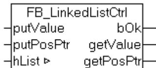
The function block FB\_LinkedListCtrl can be used to implement a linked list in the PLC project. A double-linked list is created. A linked list allows values (known as nodes) to be stored. It is possible to iterate the list from the back to the front or the other way. Nodes can quickly be added or deleted.
