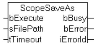
The function block "ScopeSaveAs" allows a Scope View Configuration Project (\*.scp ) to be saved under the specified file name. Internally, an instance of the ADSWRITE function block is called.
