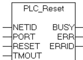
The "PLC\_Reset" function block can be used to reset a PLC run-time system. When the PLC is reset, the PLC variables are filled with their initial values, and the execution of the PLC program is stopped. Internally, an instance of the ADSWRTCTRL function block is called.
