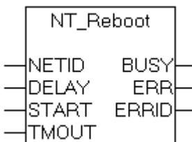
The Windows NT operating system can be restarted with the aid of the "NT\_Reboot" function block. The function largely corresponds to the Restart command on the Windows taskbar. A delay before execution of the Restart command can be defined via the DELAY parameter. Internally, an instance of the ADSWRTCTRL function block is called.
