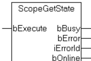
The function block "ScopeGetState" allows the state of the Scope View to be determined. If the Scope View is currently in the online state, the bOnline output is set. Internally, an instance of the ADSREAD function block is called.
