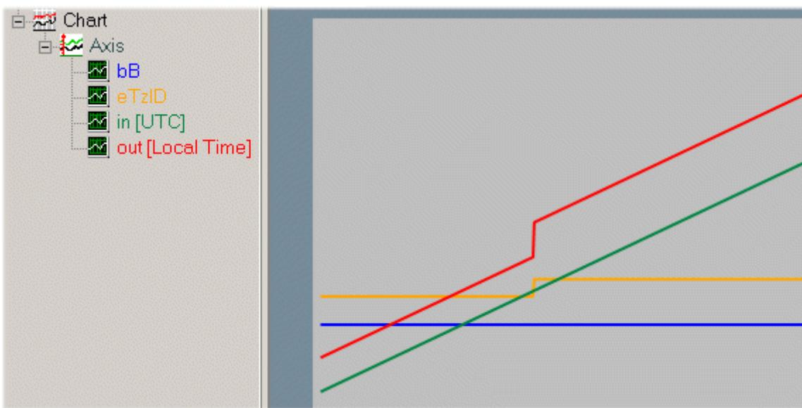
The UTC input time (green) is continuous. The local time (green) jumps forward. The local time: **2h:59m:59s:999ms..** is directly followed by: **3h:00m:00s:000ms..**. The time zone ID (orange) changes from *eTimeZoneID\_Standard* (standard time) to *eTimeZoneID\_Daylight* (daylight-saving time).
