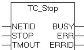
The function block "TC\_Stop" can be used to stop the TwinCAT system. The function corresponds to the Stop command on the TwinCAT system menu (on the right of the Windows taskbar).
