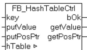
The hash table can be used as an efficient tool for finding individual data element among a larger number of data elements. The data objects must have a unique key. The key enables the data objects to be identified unambiguously and found quickly in the table.
