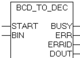
The "BCD\_TO\_DEC" function block allows numbers in BCD to be converted to decimal format. The BCD number to be converted is checked for the reliability of the values.
