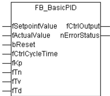
The function block represents a simple discrete PID element.
