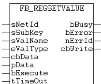
The System registration is a hierarchical structured tree. A node in the tree is called key. Each Key again can contain SubKeys, and Values.
