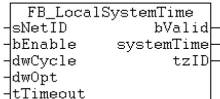
In some applications the local Windows system time is synchronized via the SNTP time server or a radio clock. The local Windows system time (the local Windows system time is displayed in the task bar) often has to be used in the PLC (e.g. for time stamp log messages to the HMI). For such applications the [FB\\_LocalSystemTime](#) function block can be useful.
