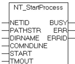
The "NT\_StartProcess" function block can be used to start a Windows application from the PLC. Internally, an instance of the ADSWRITE function block is called. The function block can also be used to run applications on a remote PC.
