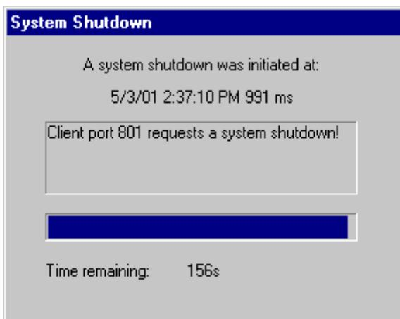
Only after the delay time has elapsed is the operating system shut down. During this time, the shutdown process can be interrupted from the PLC with the aid of the "NT\_AbortShutdown" function block.
