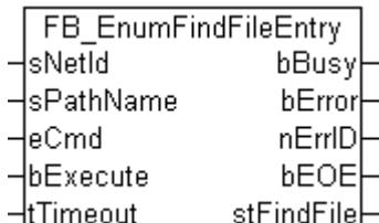
This function block searches a directory for a file or a subdirectory whose name is similar to the specified name. Any entries found can be read individually. See also description of the [FB\\_EnumFindFileList \[▶ 160\]](#) function block. The input parameter [eCmd](#) is used for navigating through the list of entries. The [eCmd](#) input determines whether the first or the next input is read, for example.
