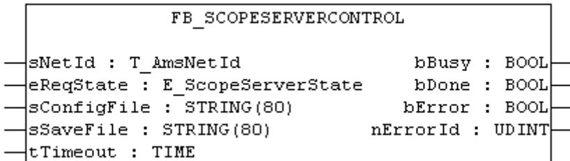
The function block "FB\_ScopeServerControl" enables the PLC to collect data for subsequent display with TwinCAT Scope View 2.
