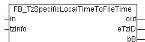
The function block converts the local time (file time format) to UTC time (file time format), considering the specified time zone information. The function block [FB\\_TzSpecificLocalTimeToSystemTime \[▶ 183\]](#) has similar functionality but uses a different time format (structured system time format).
