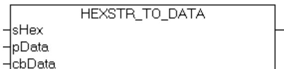
The function converts a hexadecimal string into binary data and returns the number of successfully converted data bytes as result. Only spaces may be used as separators in the hexadecimal string to be converted. Lower and upper case letters are permitted as hex characters. In the event of an error or an illegal character the conversion is aborted and a zero length is returned as result.
