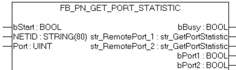
When called, this module supplies the statistical data for the ports of a PROFINET device.
