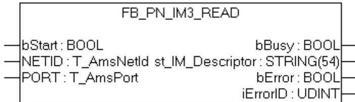
Using this function block the PROFINET controller reads all I&M3 data (Identification & Maintenance) from a device referenced via the *Port* input.
