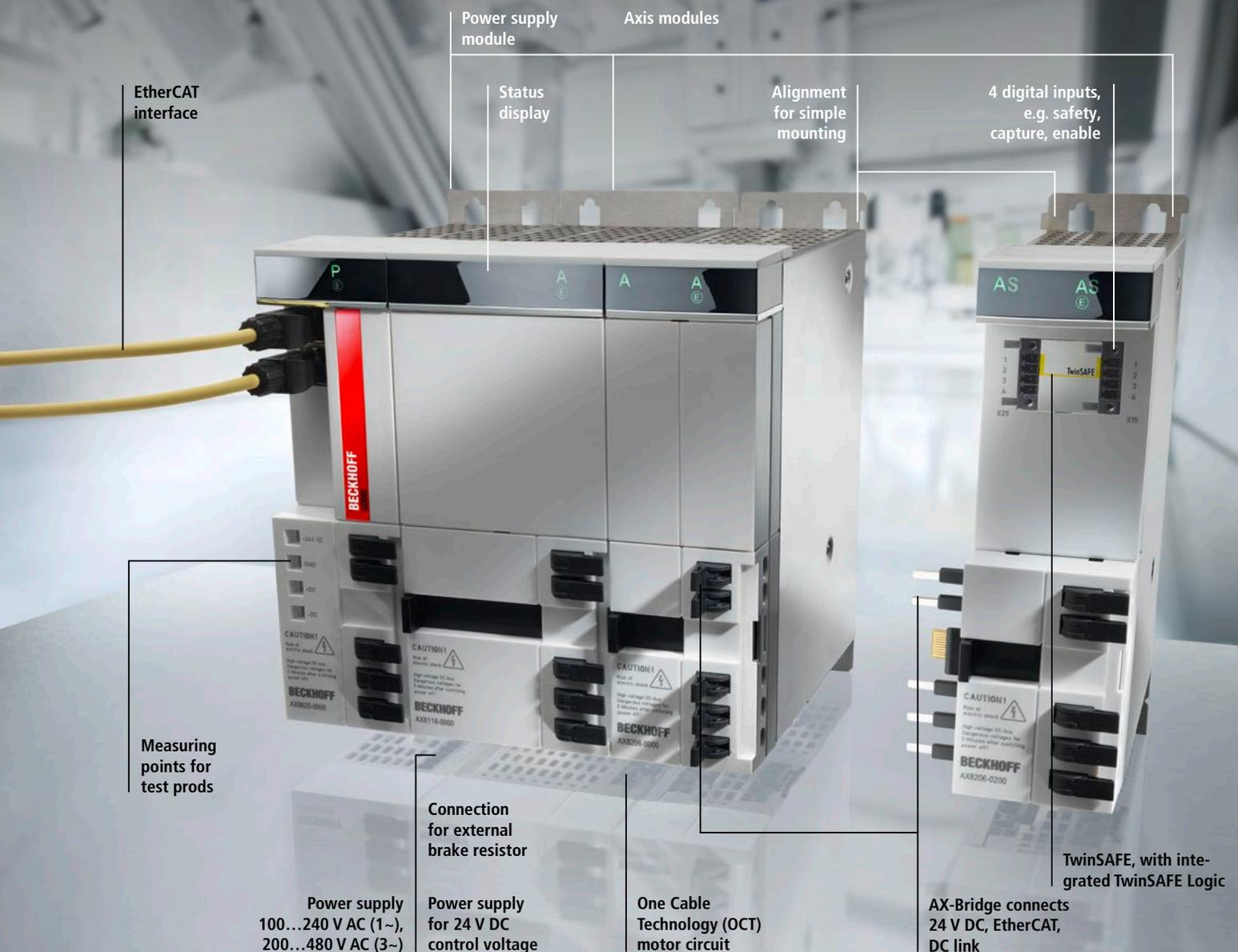
With the AX8000 multi-axis servo system, you benefit from maximum flexibility: Power supply, axis modules and other optional modules can be combined as needed for all areas of application. All requirements are covered – without the need for further components or any hidden costs. The power supply
