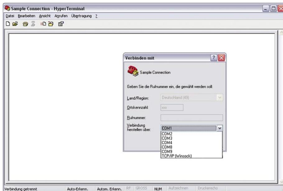
Fig. 3 Access to the virtual COM port through applications/programs (e.g. HyperTerminal)
